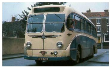
The Mark 3 reverted to the single metal strip around the "tank" moulding. This is PSUC1/2 Tiger Cub HFR 603, new to W C Standerwick in 1954 and shown here with its second operator, Butter of Childs Ercall. Standerwick's parent company, Ribble, had a similar batch. (G Lumb via E A Wain).
