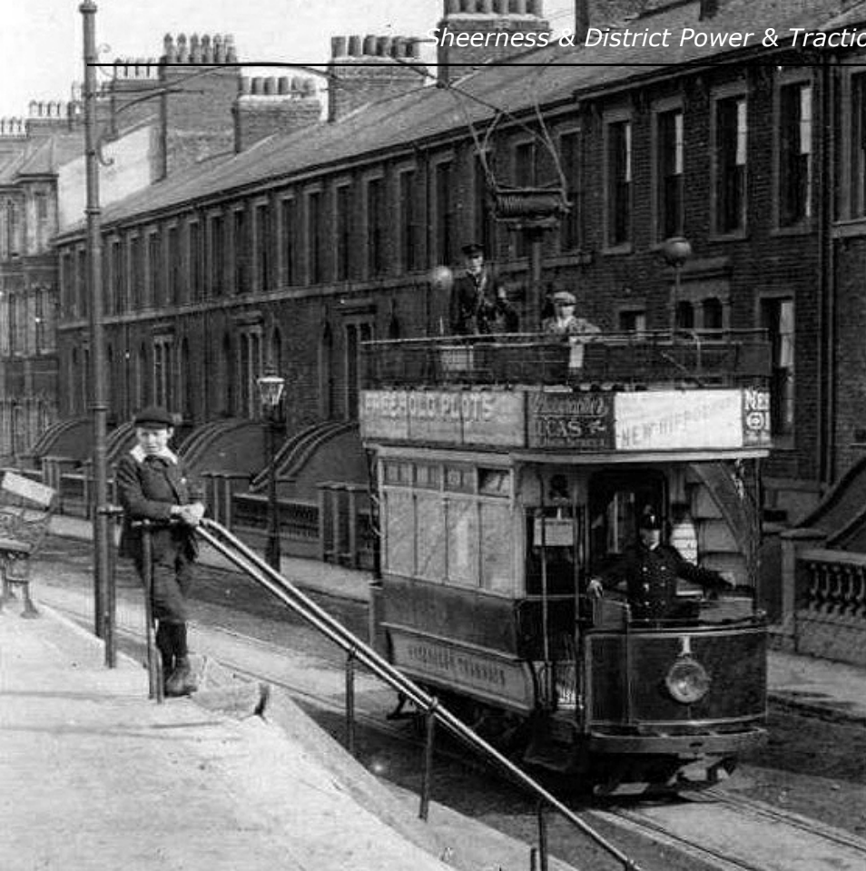
Car No. 1, dating from 1903, poses for a photograph on Marine Parade, along with an interested young boy. It clearly shows the unique bow collector employed by the tramway. The car was built by Brush on Brush trucks and seated 50. (LTHS collection).
