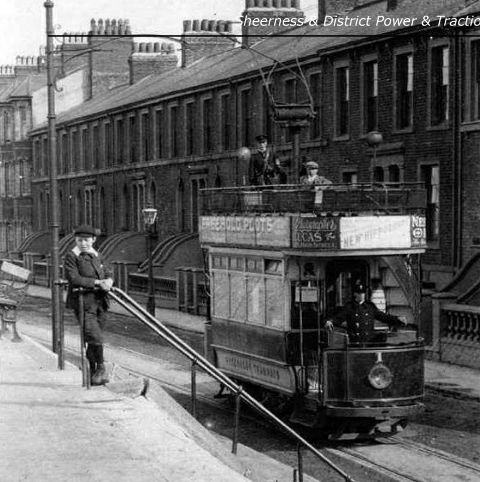
Car No. 1, dating from 1903, poses for a photograph on Marine Parade, along with an interested young boy. It clearly shows the unique bow collector employed by the tramway. The car was built by Brush on Brush trucks and seated 50. (LTHL collection).
