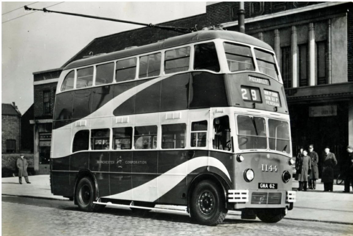
No. 1144 (GNA62) dating from 1940 was a Crossley TDD4 with Crossley 54-seat bodywork on MCCW frames. (GEC collection - courtesy David Beilby).
