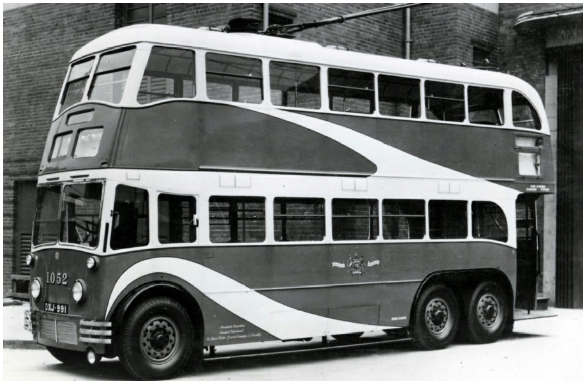
No. 1052 (DXJ991) was one of the first batch of 1938 Crossley TDD6 trolleybuses with Crossley 68-seat bodywork, seen here before delivery sporting the 'streamline' livery. It was withdrawn in 1955. (GEC collection - courtesy David Beilby).
