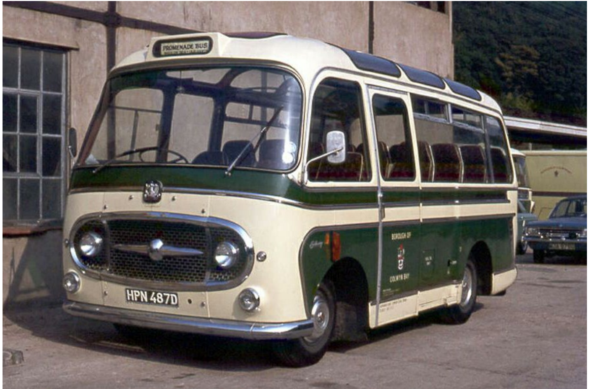
By 1968 Colwyn Bay had dispensed with fleet numbers. HPN487D was a 1966 Bedford J2SZ10 with Plaxton Embassy 20-seat coachwork. (David Everett from the John Kaye collection).
