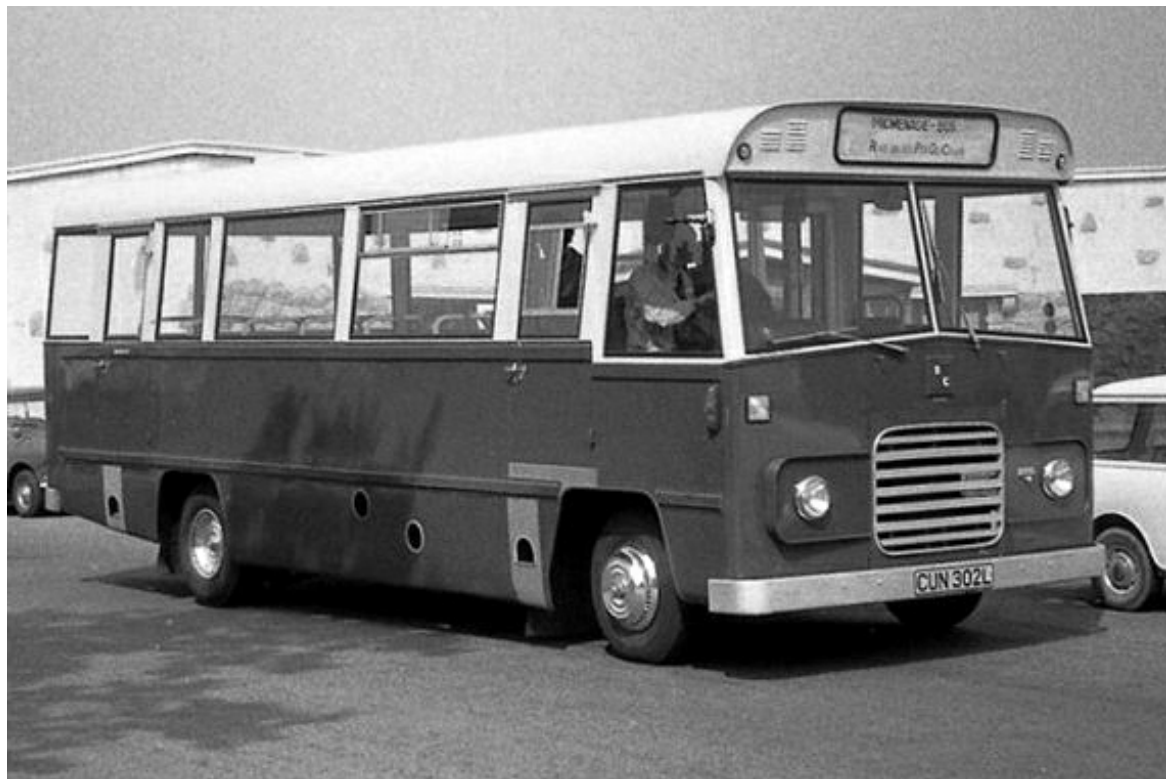
CUN302L a 1973 Bedford VAS5 with Strachan 28-seat bodywork seen here operating the Promenade service. (LTHL collection).
