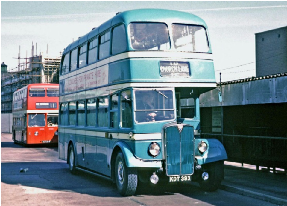
KDT393 was only 4 years old when acquired in 1955 from Doncaster Corporation. It was an AEC Regent III with Roe 56-seat bodywork, withdrawn in 1967.(LTHS - photographer unknown).
