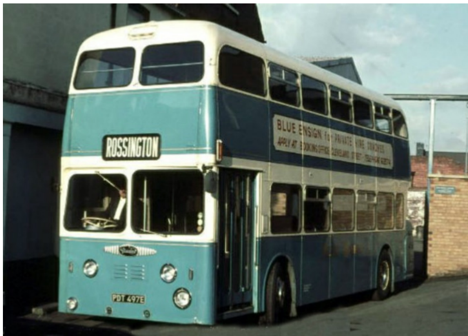
Blue Ensign's first rear-engined bus was this Daimler CRG6LX (FDT497E) with Roe 78-seat bodywork that passed to South Yorkshire PTE as their No. 1328 in 1978. (Bruce Tilley).
