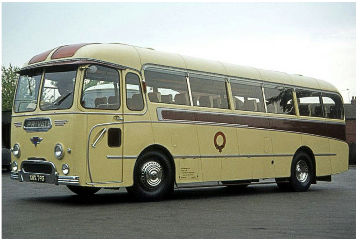
No. 40 (XWX795), a 1959 AEC Reliance with Roe 41-seat coachwork, seen here at Felix's Park Lane depot in 1973. (John Stringer).
