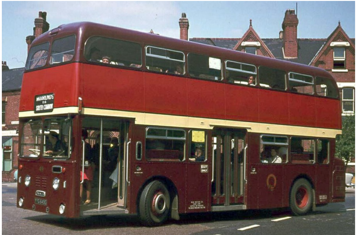
No. 49 (YYG649G) was Felix Motors' first rear-engined vehicle. It was a 1969 Daimler CRG6LX with Roe 74-seat dual door bodywork. (John Kaye).
