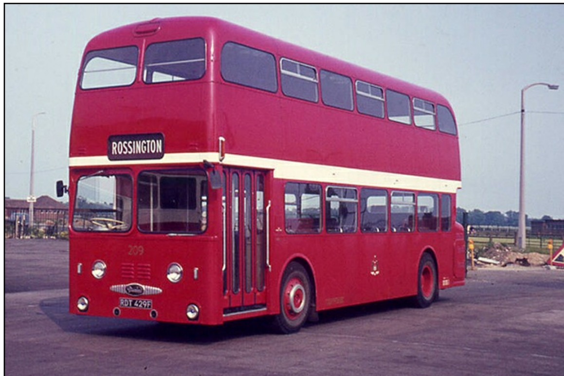
No. 209 (RDF429F) was one of Doncaster's first rear-engined double-deckers. It was a 1967 Daimler CRG6LX with Roe H44/34F bodywork, seen here in Leicester Street garage in June 1968. (John Kaye).
