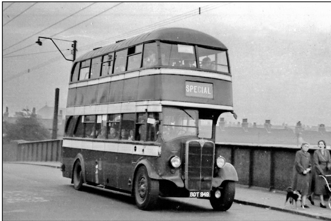
No. 57 (BDT948), a 1941 AEC Regent with Roe 54-seat bodywork that gave 20 years of service before being withdrawn in 1961. (LTHL collection).
