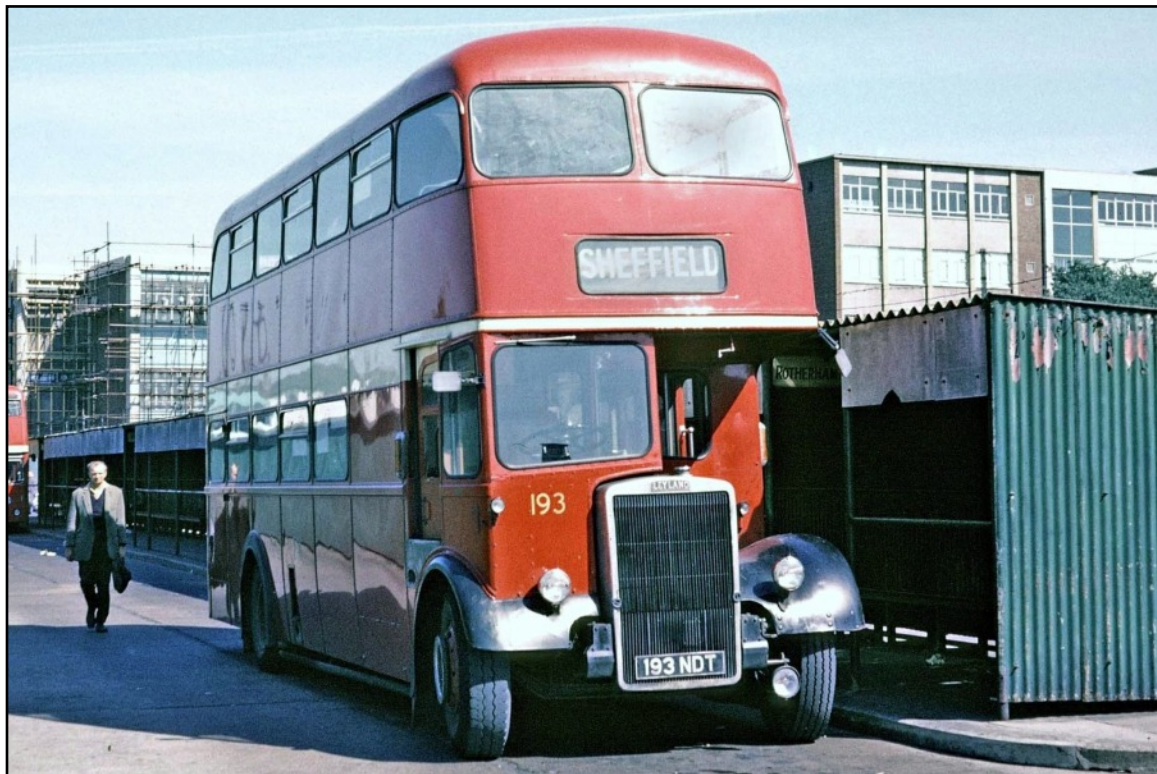
No. 193 (193NDT), a 1963 Leyland P3/4 was fitted with a Roe 62-seat ex-trolleybus body, converted to half cab, from new. (LTHL collection).
