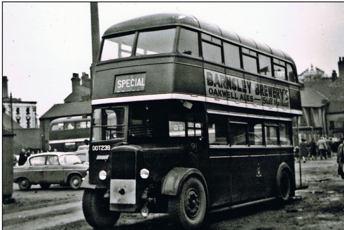
1946 Daimler CWA6 No. 91 (DDT239) with Roe 56-seat bodywork, withdrawn in 1963. (LTHL collection).
