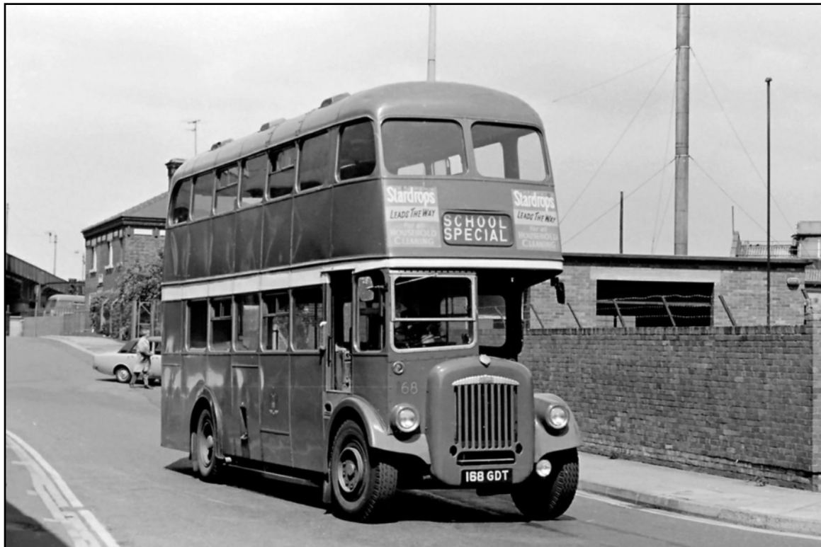
No. 168 (168GDT), a Daimler CVG6 new in 1962 with 1959 Roe 62-seat body from trolleybus No. 386, rebuilt to half-cab layout. (LTHL collection).
