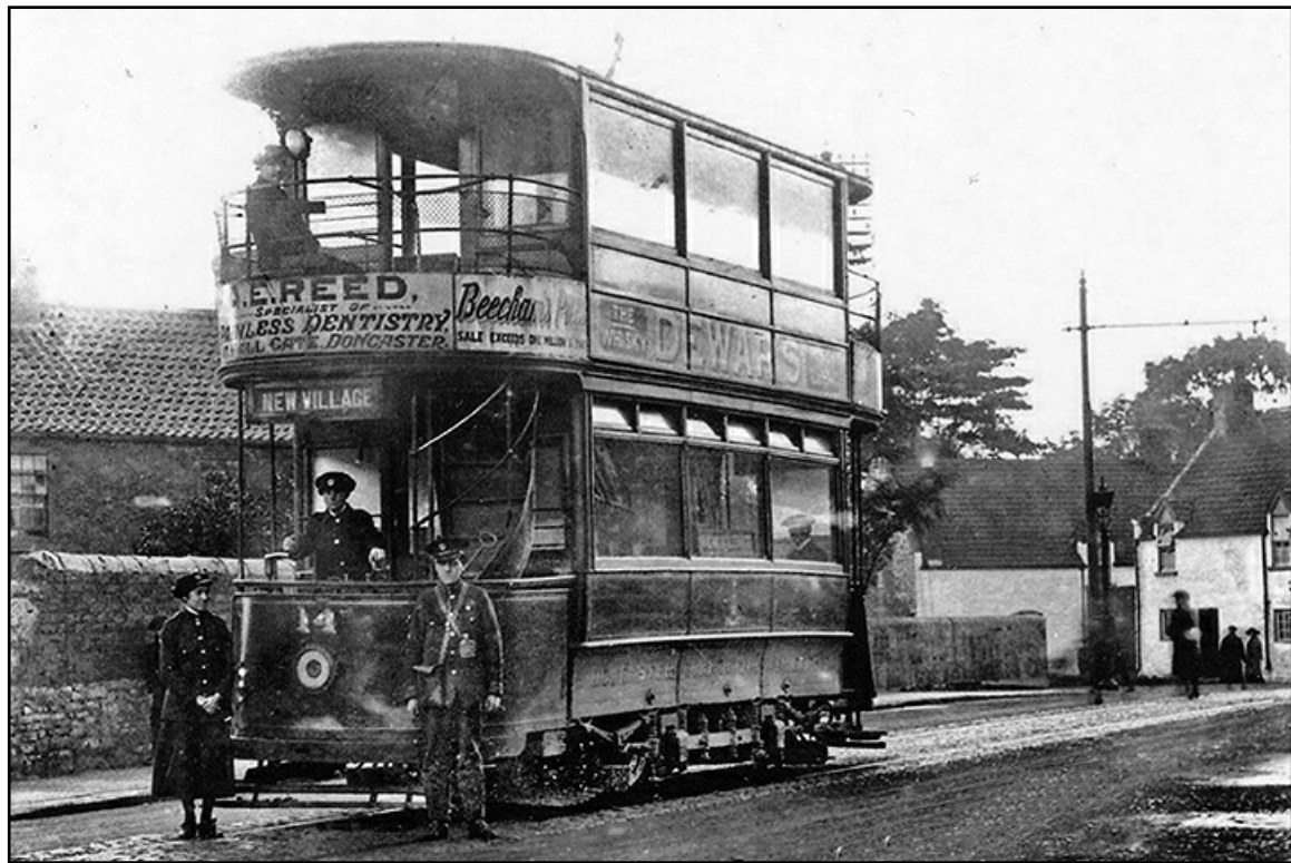
Car No. 14, built by ERTCW in 1902, was fitted with its Dick, Kerr top cover in 1913 and, although looking very battered here during World War 1, it survived until 1930. (LTHL collection).
