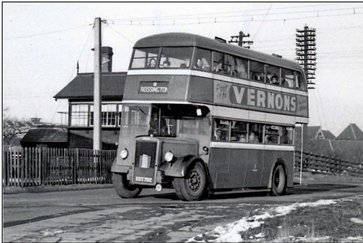
No. 93 (EDT702) was an all-Leyland PD2/1 dating from 1947. It was fitted with a 1955 Roe-built ex-trolleybus body in 1963. (LTHL collection).
