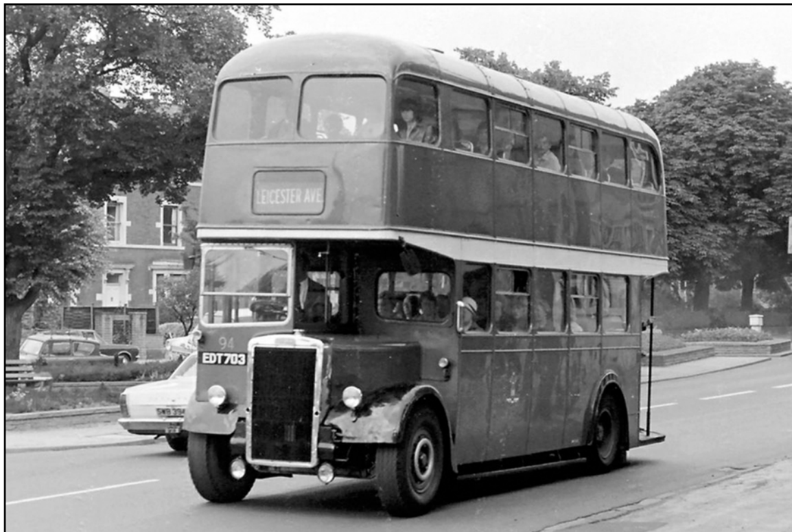
No. 94 (EDT703), a 1947 Leyland PD2/1, originally with a Leyland 56-seat body (see previous page) was re-bodied in 1963 with this 1955 Roe body from trolleybus No. 393. (LTHL collection).
