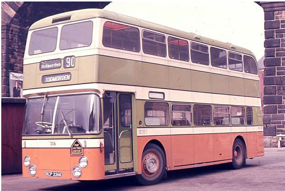
Calderdale JOC No. 306 (RCP336K), a 1972 Daimler CRG6LX with Northern Counties 74-seat bodywork. (Alan Hall).
