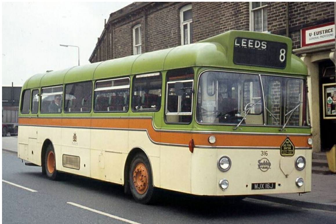
Halifax JOC No. 316 (MJX16J), a 1970 Seddon RU with Plaxton Derwent 45-seat dual purpose body. Seen here in April 1971 en route to Leeds, it passed to Calderdale JOC in September retaining its fleet number. (John Kaye).
