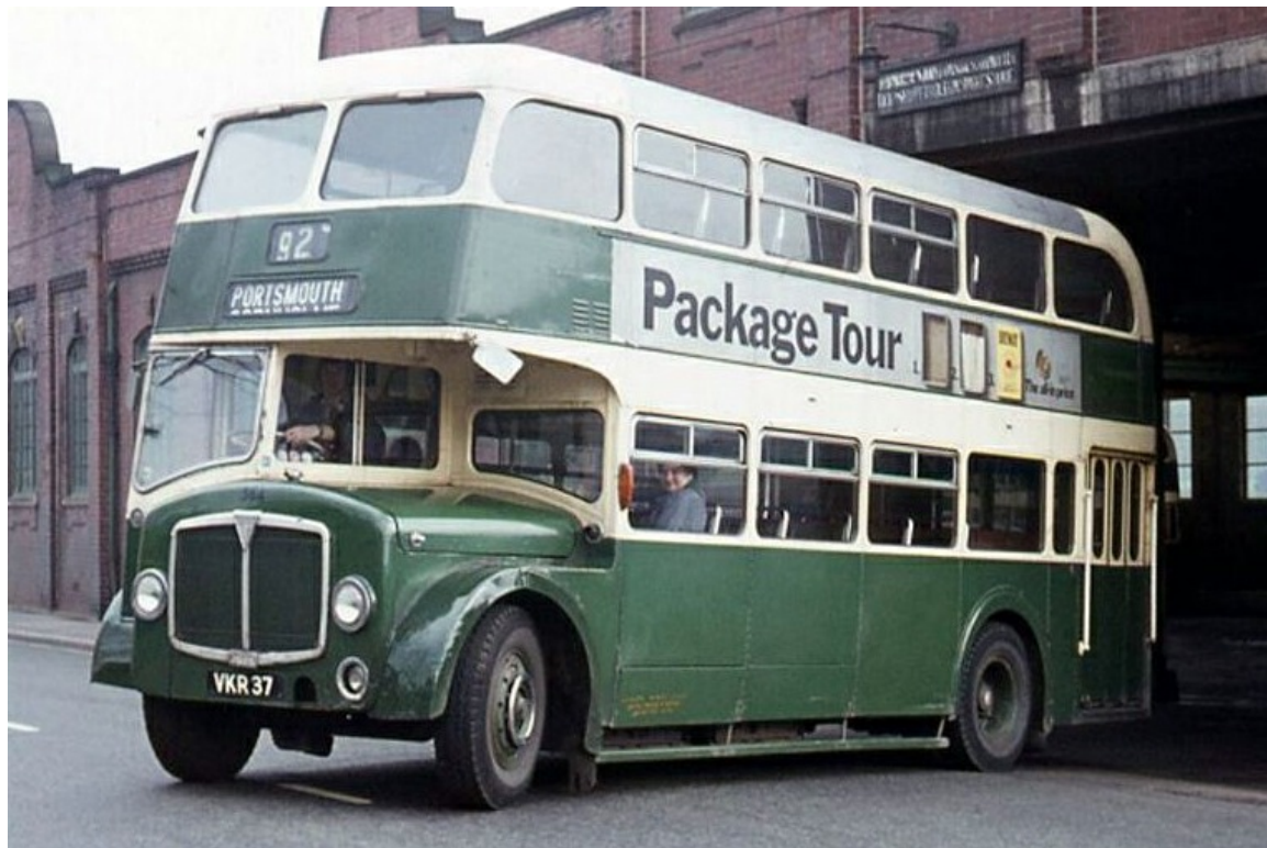
No. 364 (VKR37) was an ex-Maidstone & District AEC Regent V with Park Royal lowbridge bodywork and is seen leaving Todmorden's Millwood Garage in April 1972. (John Kaye).
