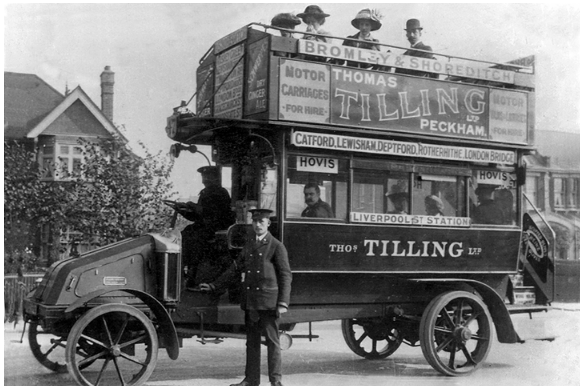
The Tilling-Stevens TTA1 model was introduced into Tillings' London services from 11th June 1911. The new petrol electric bus weighed 2 tons 8 cwt. was designed to carry 2 ton loads and employed a 4.3 litre 4 cylinder engine of 30 hp. (LTHL collection).
