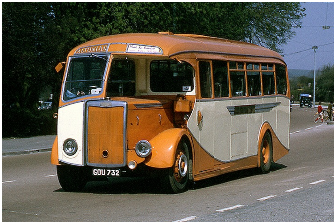
Dating from 1949 this is a post war Tilling-Stevens dropped frame K6LA7 with conventional design and pre-war style radiator with a slightly curved profile, seen here with Altonian Coaches it is now in preservation. (Roger Cox).
