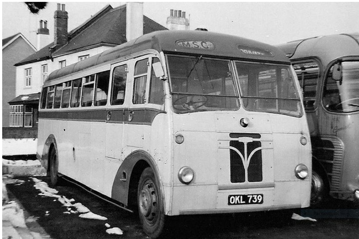
In 1950 Tilling-Stevens introduced the L4MA8, that was essentially an extended version of the L6PA7 chassis with a wheelbase of 18 ft 7½ins allowing the fitment of full fronted 30ft by 8ft bodywork. (Barry Nunn).
