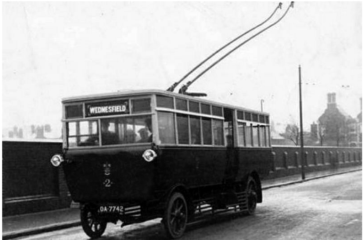
Tilling-Stevens' best trolleybus customer was Wolverhampton Corporation which took thirty two between 1923 and 1926, all with Dodson bodywork based upon the TS6 chassis in which the engine and dynamo were replaced by BTH electrical equipment. (LTHL collection).
