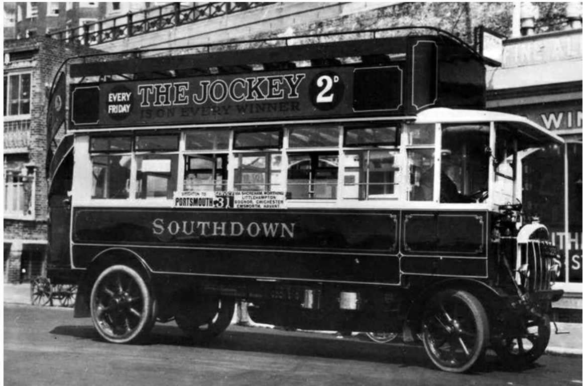
A Southdown Motor Services Tilling-Stevens TS6. The TS6 was a forward control machine of 1921 for 5 ton loads/up to 64 passengers, and was usually powered by the 5.7 litre engine of the TS3A. (LTHL collection).
