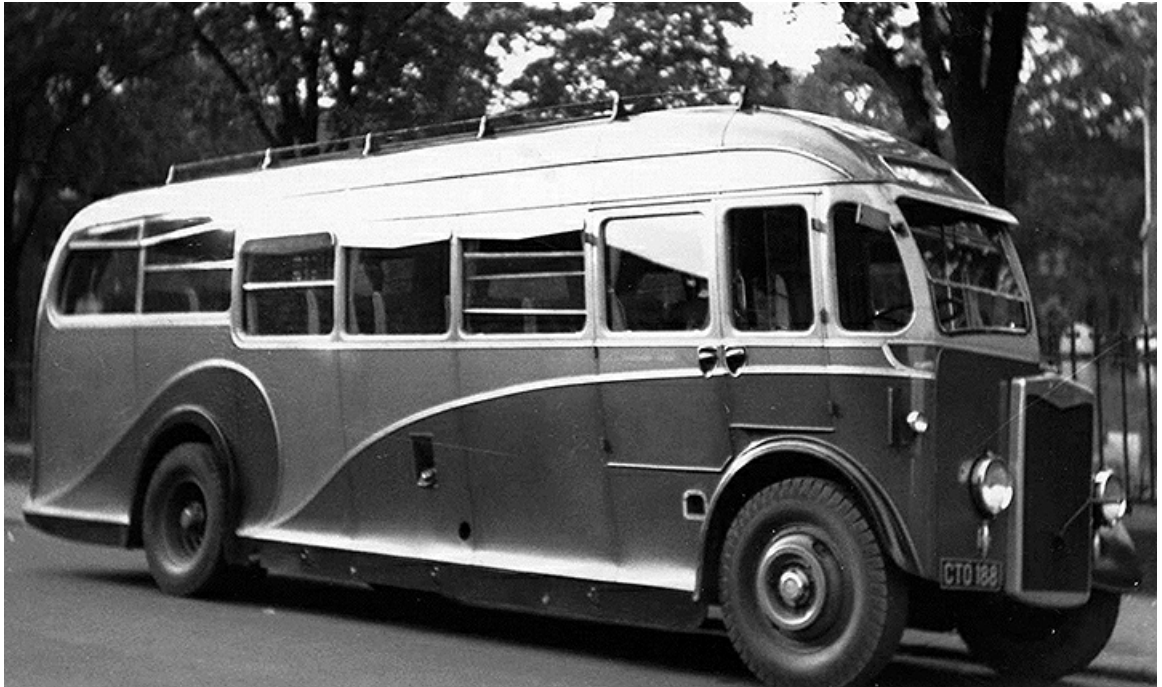
A 1936 HA39A7 model, a single deck 7 ton chassis, that was an updated development of the proven B type. This was promoted as the 'New Express' for 32-39 seat bodies with the 5.12 litre four cylinder petrol engine, rated at 74 bhp at 2,100 rpm. (LTHL collection).
