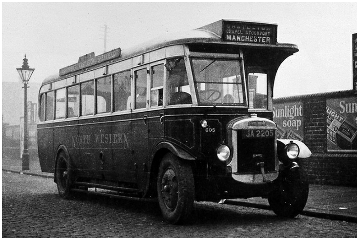
North Western B10A2, one of the lower framed B10A and B10B chassis that became the most commercially successful Tilling Stevens types. Some 2000 B9/B10 machines had been sold at home and overseas by the mid-1930's. (LTHL collection).
