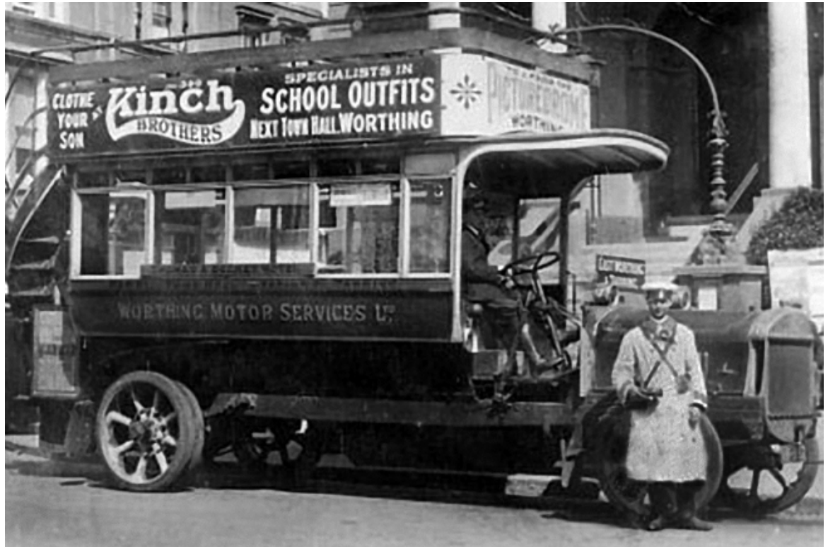
From 1914, Tilling-Stevens introduced the TS3 for 4 ton loads or up to 50 passengers. With the TS3 came the change in chassis designation from TTA to TS to reflect the name of the manufacturer rather than the major operator. (LTHL collection).
