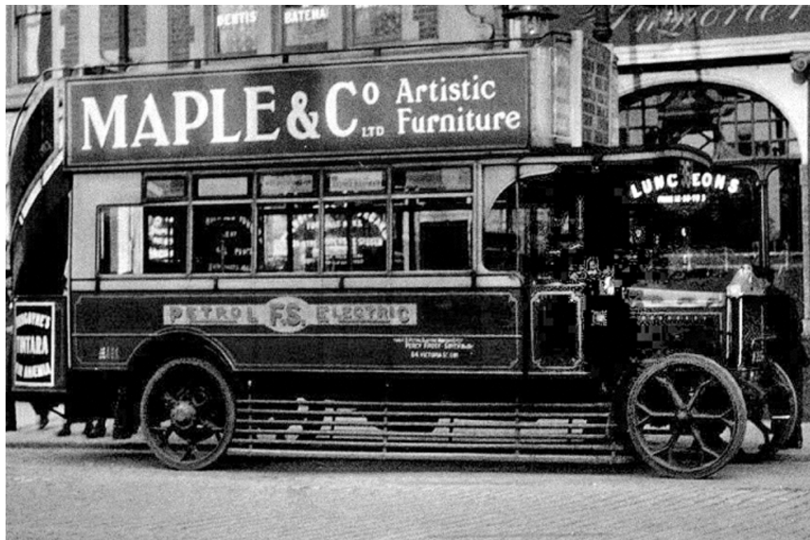
Percy Frost-Smith's fleet of F-S buses, despite employing well proven components such as four cylinder 6.23 litres White & Poppe engines developing 40hp at 1,000 rpm, the six examples constructed proved woefully unreliable. (LTHL collection).
