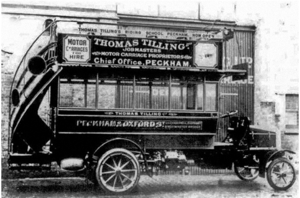
The pioneer Hallford-Stevens that utilised an electric motor at each rear wheel, a transmission system that was subsequently employed by some USA manufacturers of petrol electric chassis. (LTHL collection).
