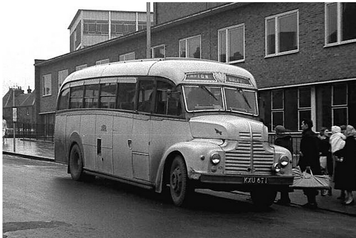
K71 (KXU671), a 1950 Leyland CP01 Comet with Windover 32-seat coachwork. (John Boylett courtesy John Kaye).
