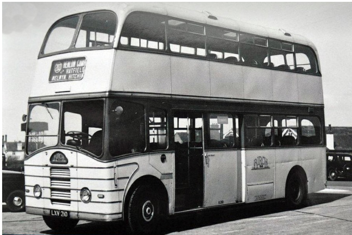
K210 (LXV210), a 1951 Guy Arab III with Willowbrook full-front 53-seat bodywork. It carried the name John Churchill. (LTHL collection).
