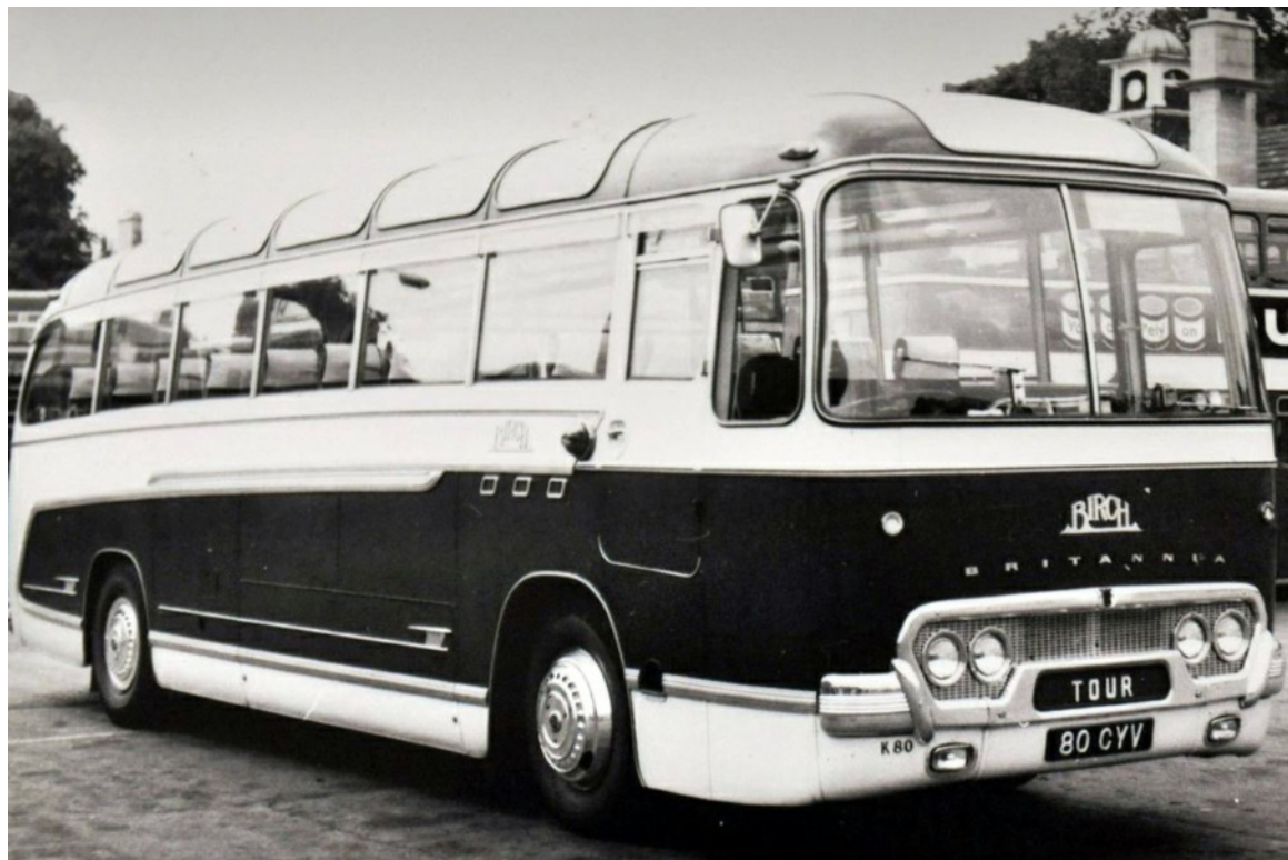
K80 (80CYV), a 1961 Leyland L2 Leopard with Duple Britannia 41-seat bodywork. (LTHL collection).
