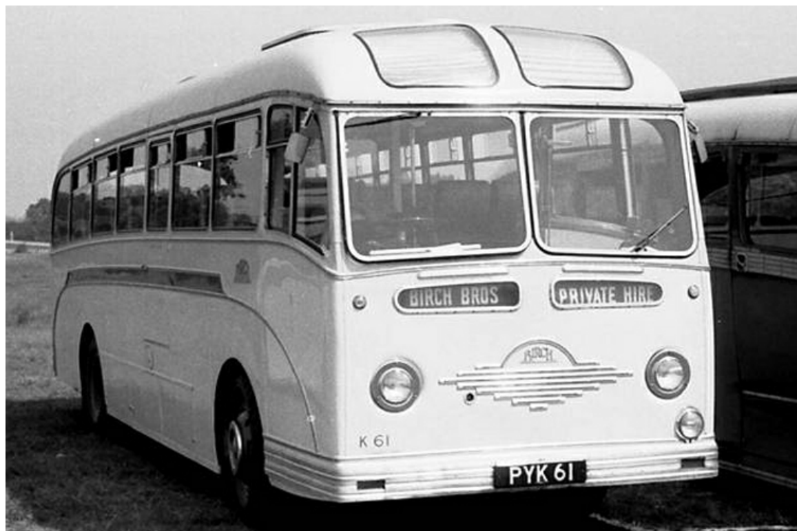
K61 (PYK61) was one of 6 Beadle-Commer TS3 rebuilds purchased in 1955 - it carried Beadle 41-seat coachwork. (John Boylett courtesy John Kaye).
