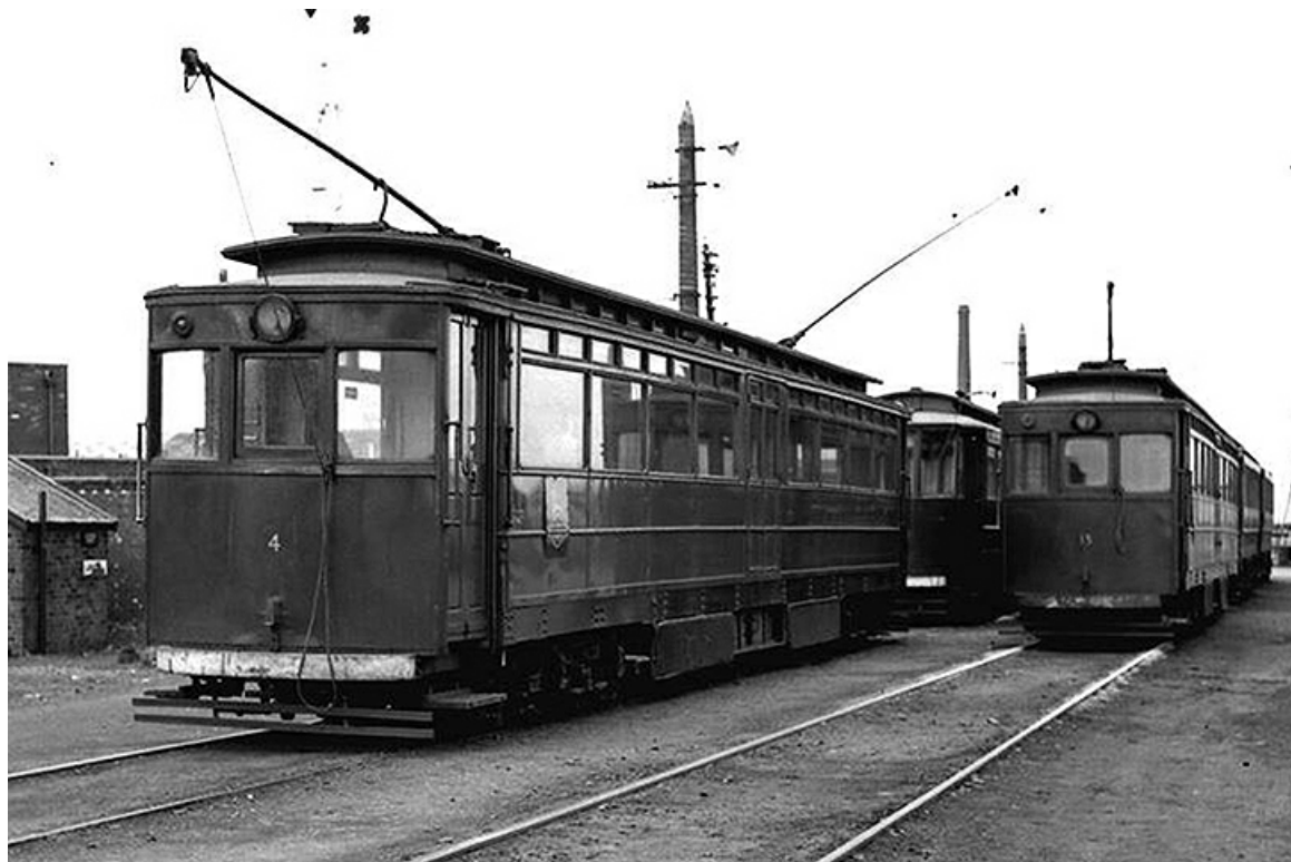
Grimsby & Immingham cars No. 4 and No. 15 at Immingham. Two of the original bogie cars, No. 4 dating from 1911 and No. 15 from 1915. No. 4 was the last tram to operate on 1st July 1961. They were 54' long and seated 72 on wooden seats. (John Kaye).
