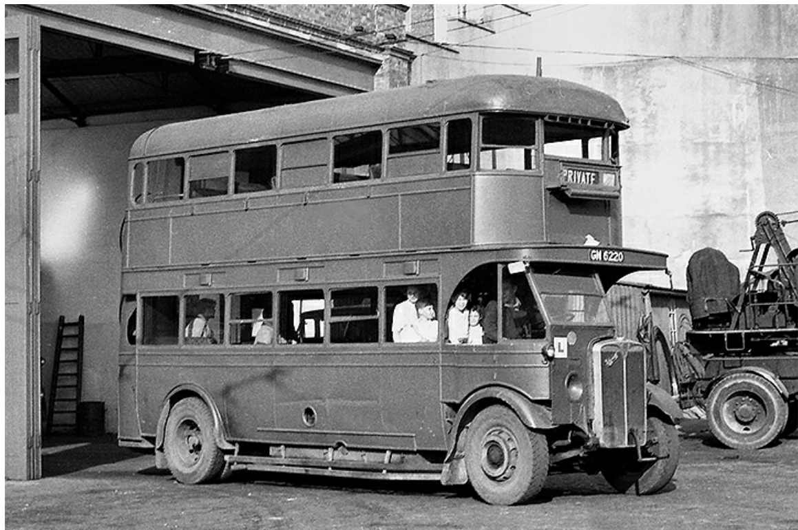
GN6220 was a 1931 AEC Regent with Dodson 52-seat open staircase bodywork, originally acquired for driver training in 1939, it was pressed into service and numbered 81, but withdrawn the following year. (Mike Morant collection).
