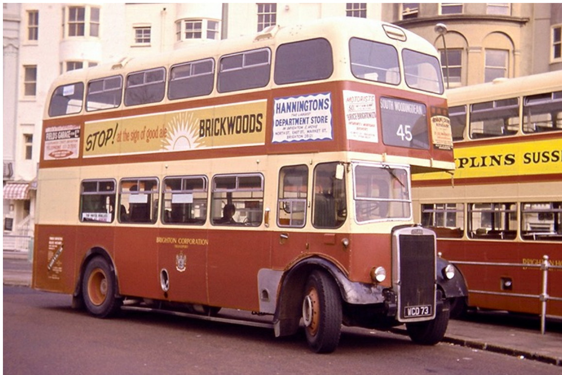
In 1959 the vehicles ordered for trolleybus replacement were Leyland PD2/37 with Weymann H33/28R bodywork. This is No. 73 (WCD73). (John Huddleston).
