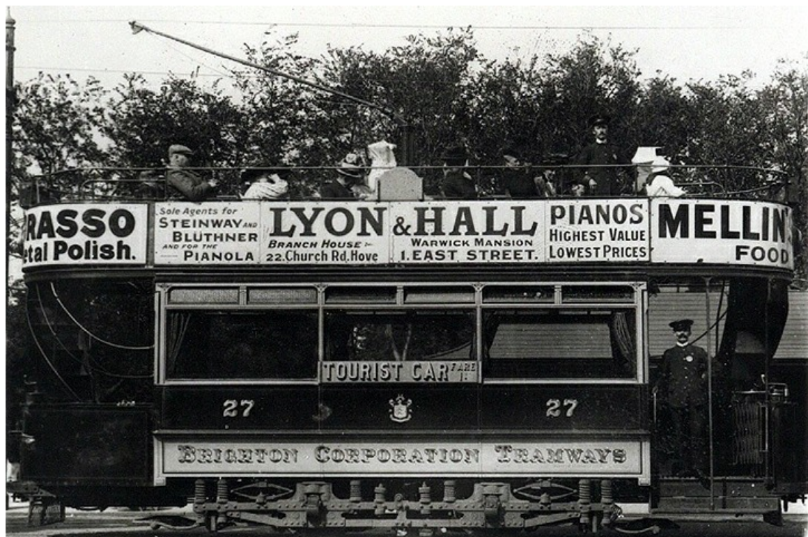
Built in 1902 by George Milnes & Company was car 27, seating 52. It was withdrawn in 1921 and replaced by a Brighton built car bearing the same number. (LTHL collection).
