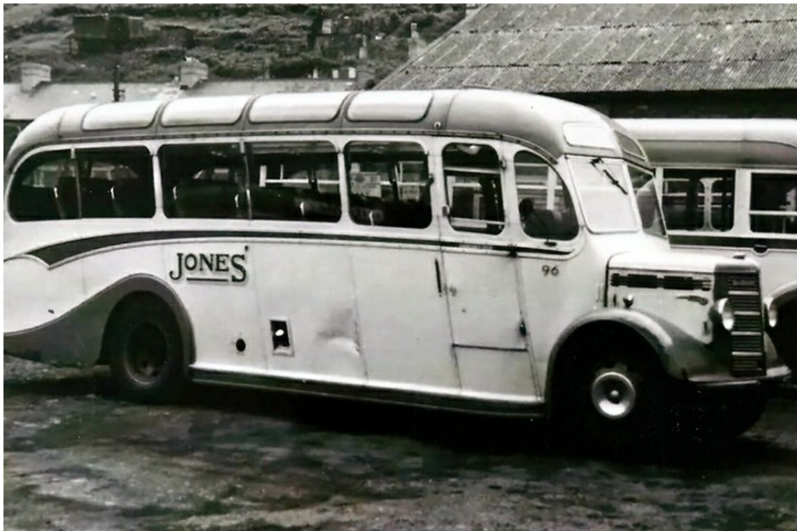
LOD533, was a 1950 Bedford OB with Duplex 29-seat coachwork, new to Princess Tours, but seen here after disposal in 1959 with Jones. (LTHL collection).
