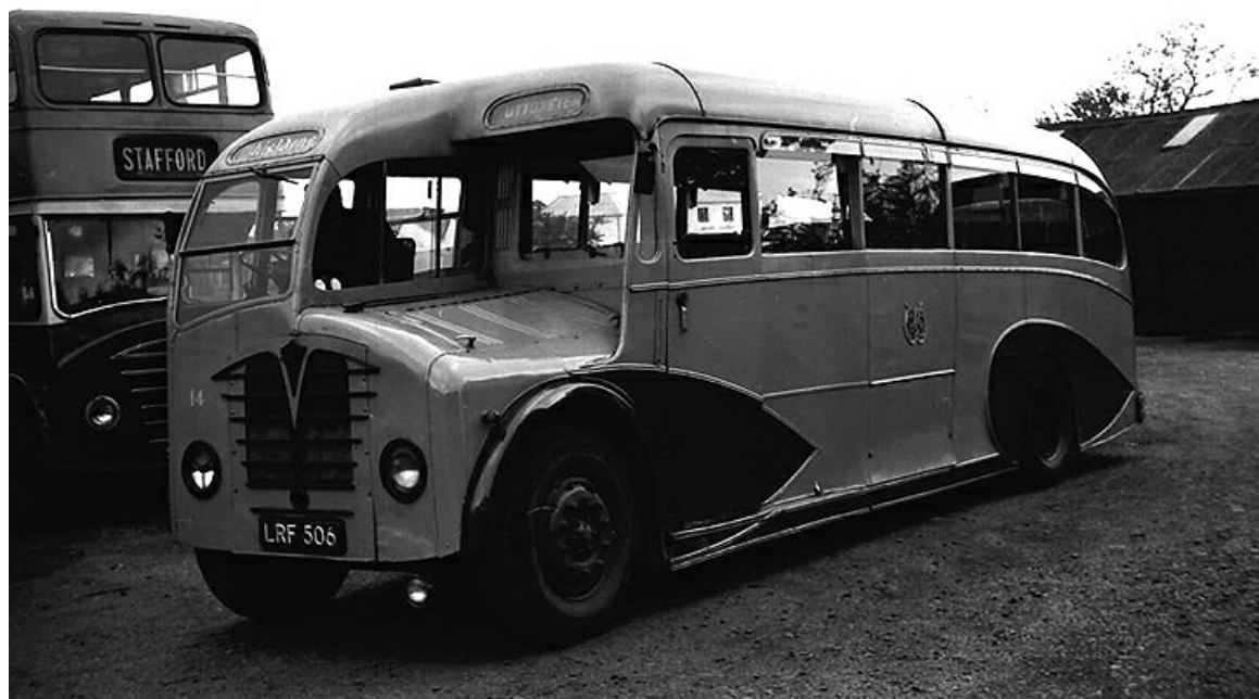
No. 14 (LRF506) was a 1947 Foden PVSC6 originally with with Eastern Counties bodywork but seen here with its 1949 Windover 33-seat coachwork. (John Boylett courtesy John Kaye).
