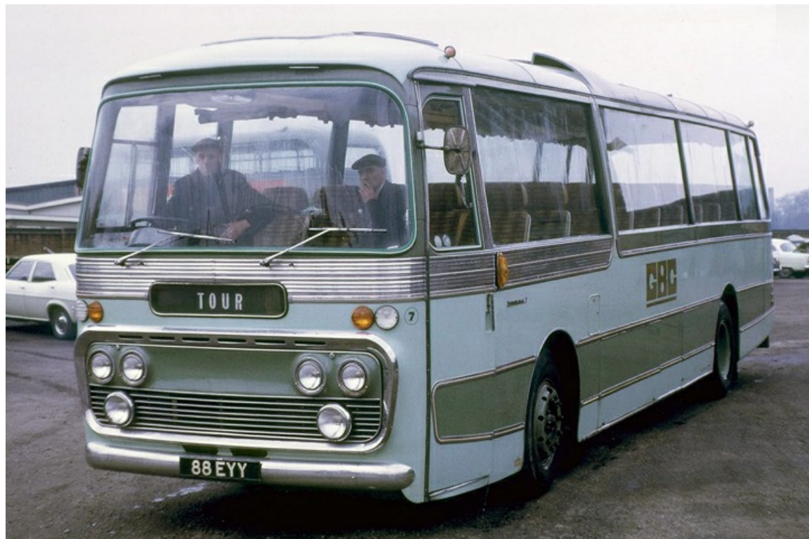
No. 7 (88EYY) was a 1963 AEC Reliance originally with Plaxton C36F bodywork but seen here after re-bodying by Plaxton to C45F before entering service with Green Bus in 1968. (Cliff Essex).
