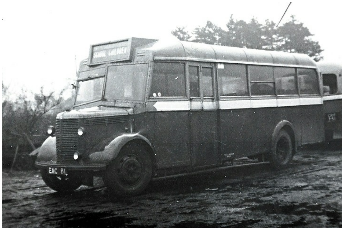
No. 5 (EAC81) was a second-hand Bedford OVB with Mulliner B32F bodywork dating from 1943 purchased in 1946. (Bus Archive).
