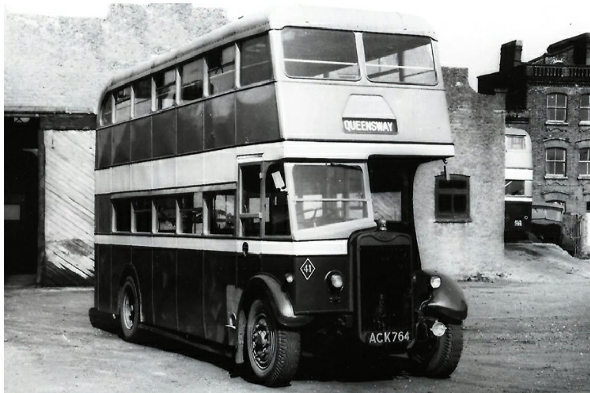
No. 41 (ACK764) came second-hand from Ribble Motor Services in 1956. Dating from 1943 it was a Guy Arab II with Northern Counties 53-seat lowbridge bodywork. (Bus Archive).
