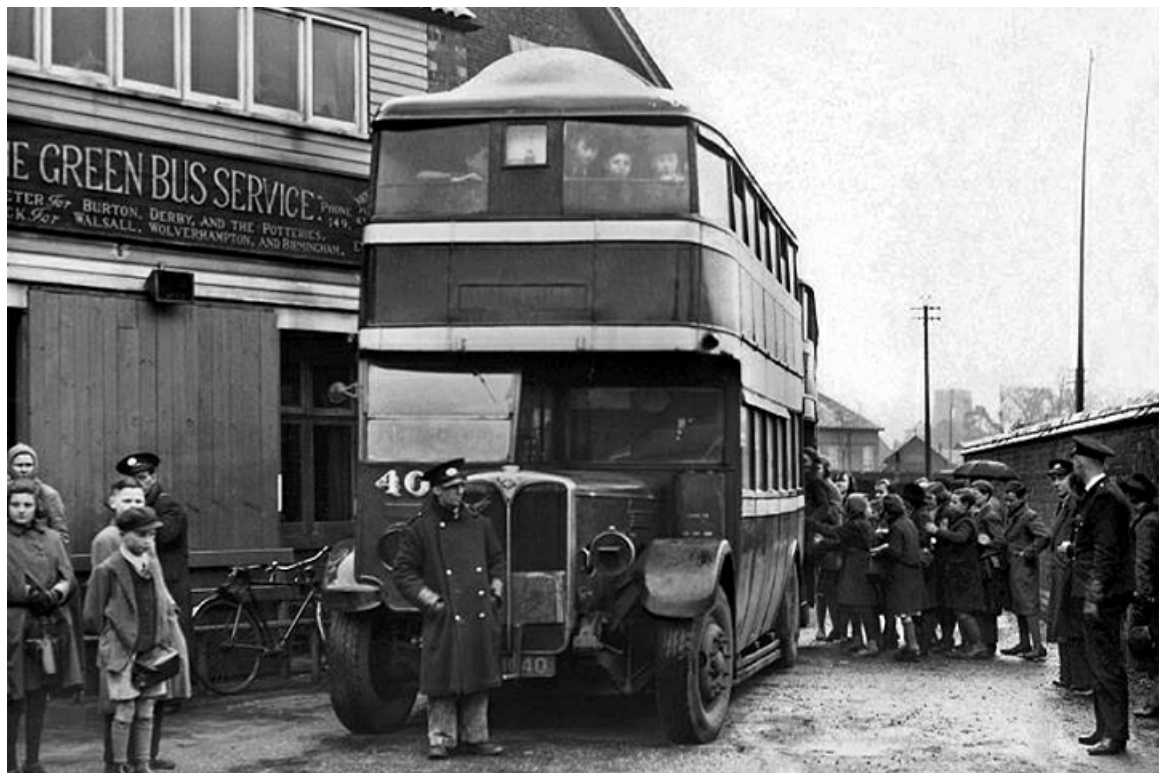
No. 40 (TV1640), a second-hand purchase from Newcastle Corporation was a 1930 AEC Regent with Park Royal H26/24R bodywork. (LTHL collection).
