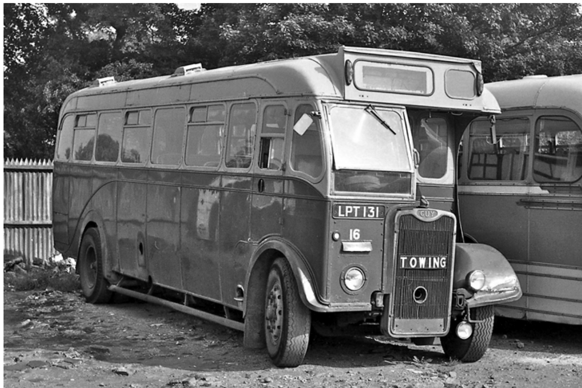
No. 16 (LPT131) was a 1950 Guy Arab III with Brush B38F bodywork, formerly in the Northern General fleet, seen here after withdrawal when in use as a towing bus. (Len Wright).
