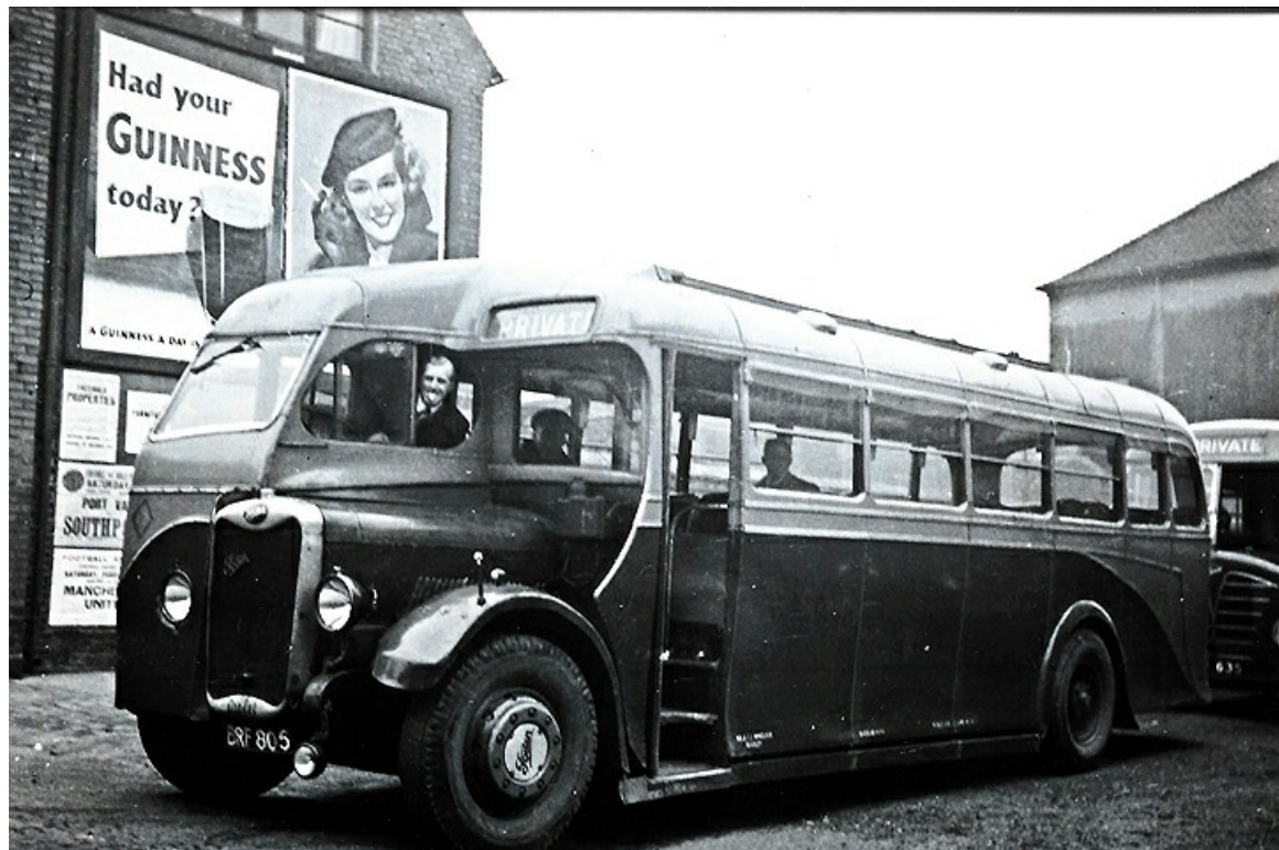
No. 7 (BRF805) was a 1933 Foden SDG6 with 31-seat Burlingham bodywork. It was re-bodied in 1949 with a second-hand ECOC 34-seat body and re-numbered 12. (Bus Archive)
