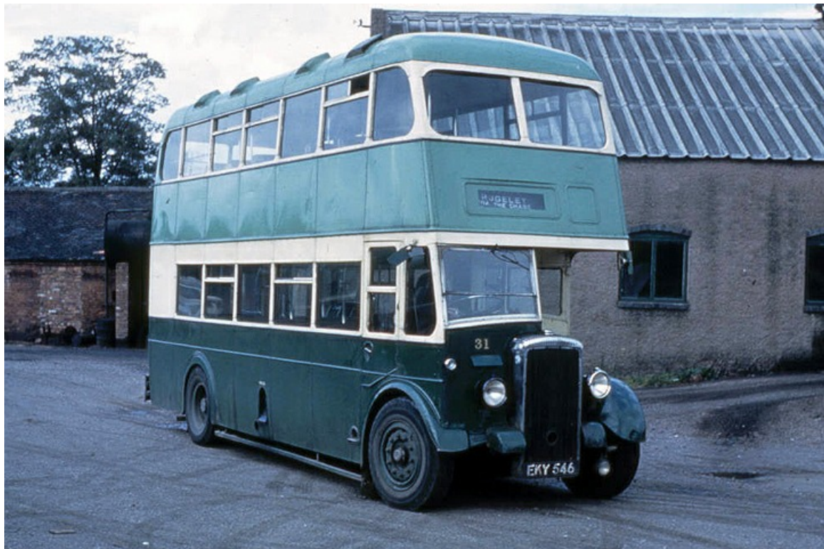
No. 31 (EKY546) was a Daimler CVD6 with Brush H33/26R bodywork that came second-hand from Bradford Corporation in 1959. (Donald Hudson).
