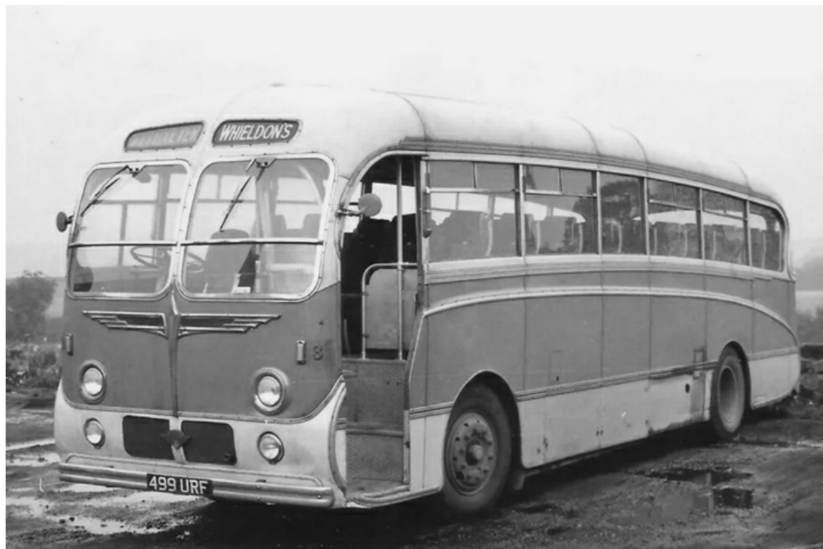
No. 3 (499URF), a 1958 Guy Arab underfloor-engined LUF with Burlingham 'Seagull' 41-seat coachwork. (LTHL collection).
