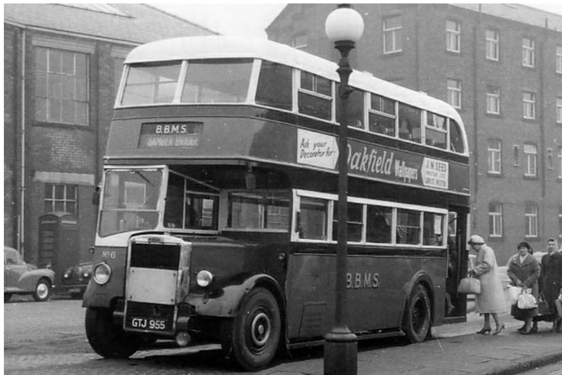
No. 6 (GTJ955) was formerly in the fleet of Corless of Coppull and was a 1947 Leyland PD1 with Leyland 53-seat lowbridge bodywork. It was fitted with platform doors in 1957. (LTHL collection via Malcolm Jones).
