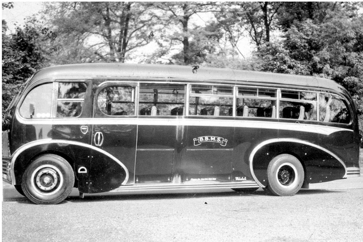
No. 2 (LTJ119) was a 1950 Leyland PS1/1 'Tiger' with Burlingham full-fronted 33-seat coachwork. (Prescott family collection).
