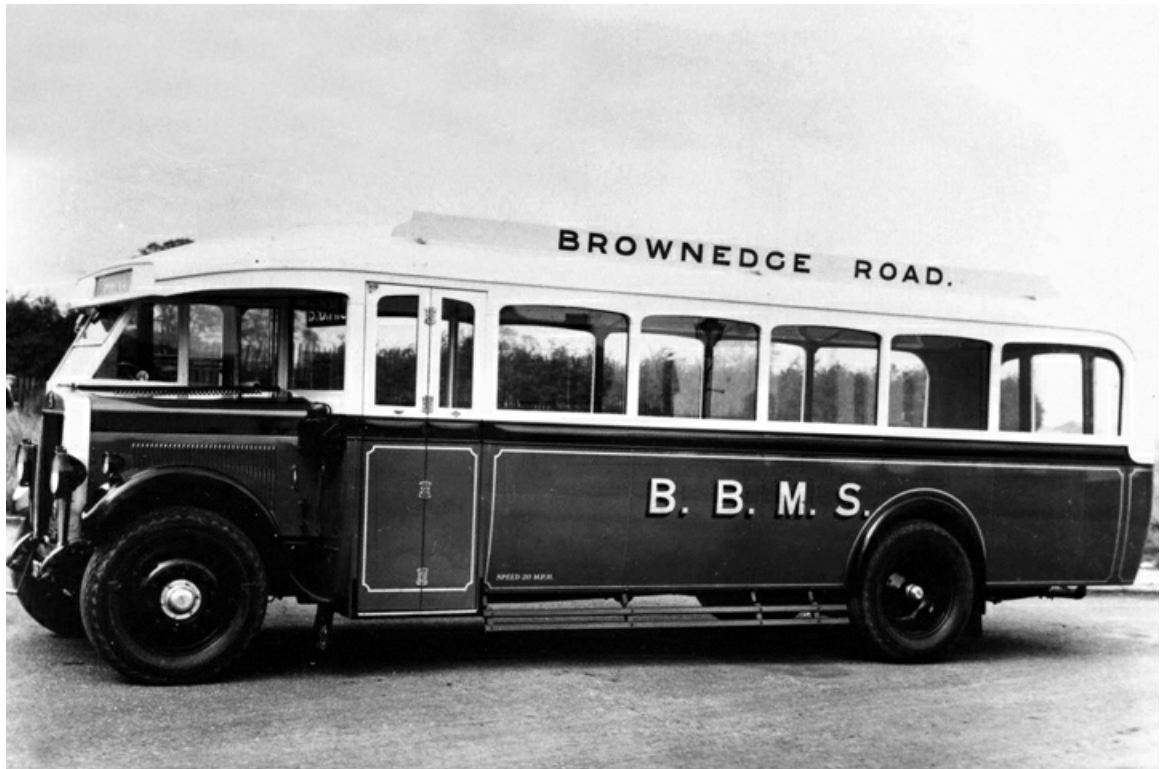
The first new vehicle for Bamber Bridge was this 1930 Leyland LT2 No. 3 (TF2693) with Leyland B32F bodywork. (Preston Digital Archive).
