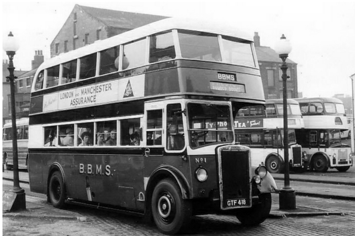
No. 1 (GTF418) was a 1946 Leyland PD1 with Leyland 53-seat bodywork, seen here in Starch House Square, Preston alongside several Scout Motor Services vehicles. (LTHL collection via Malcolm Jones).
