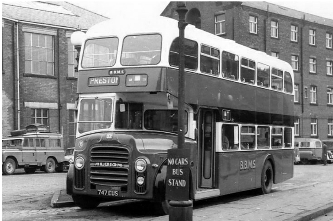
No. 6 (747EUS) was an Albion Lowlander LR1 with Alexander 72-seat bodywork, the only highbridge layout bus operated by BBMS. (LTHL collection via Malcolm Jones).
