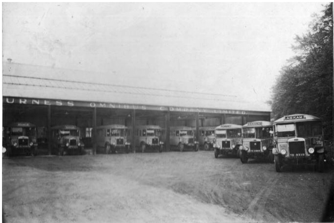
This photo was probably taken in 1928 and shows the depot at Dalton-in-Furness and some of the fleet. The vehicle on the right nearest the camera is No. 11 (TD9219) a 1927 Leyland LSC1 'Lion' with Leyland B31F bodywork. (LTHL collection).
