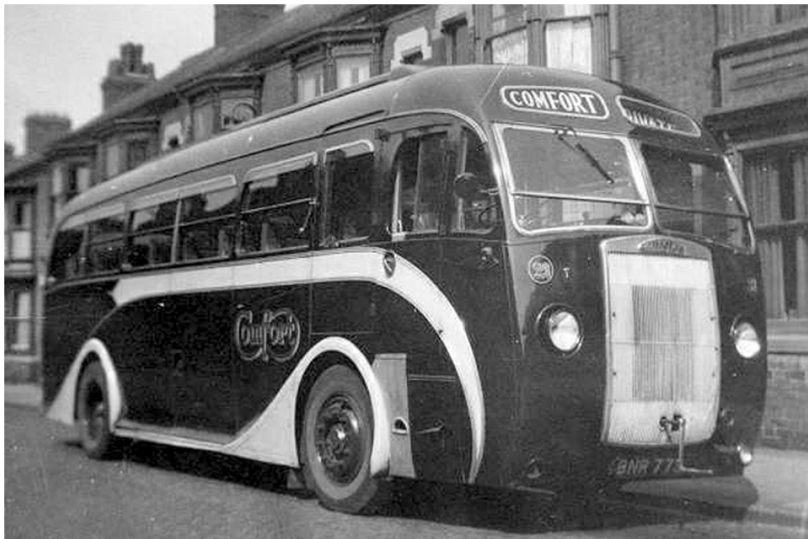
No. 21 (BNR779), a 1939 Maudslay 'Magna' SF40 with Willowbrook 36-seat dual-purpose bodywork. (LTHL collection/unknown).
