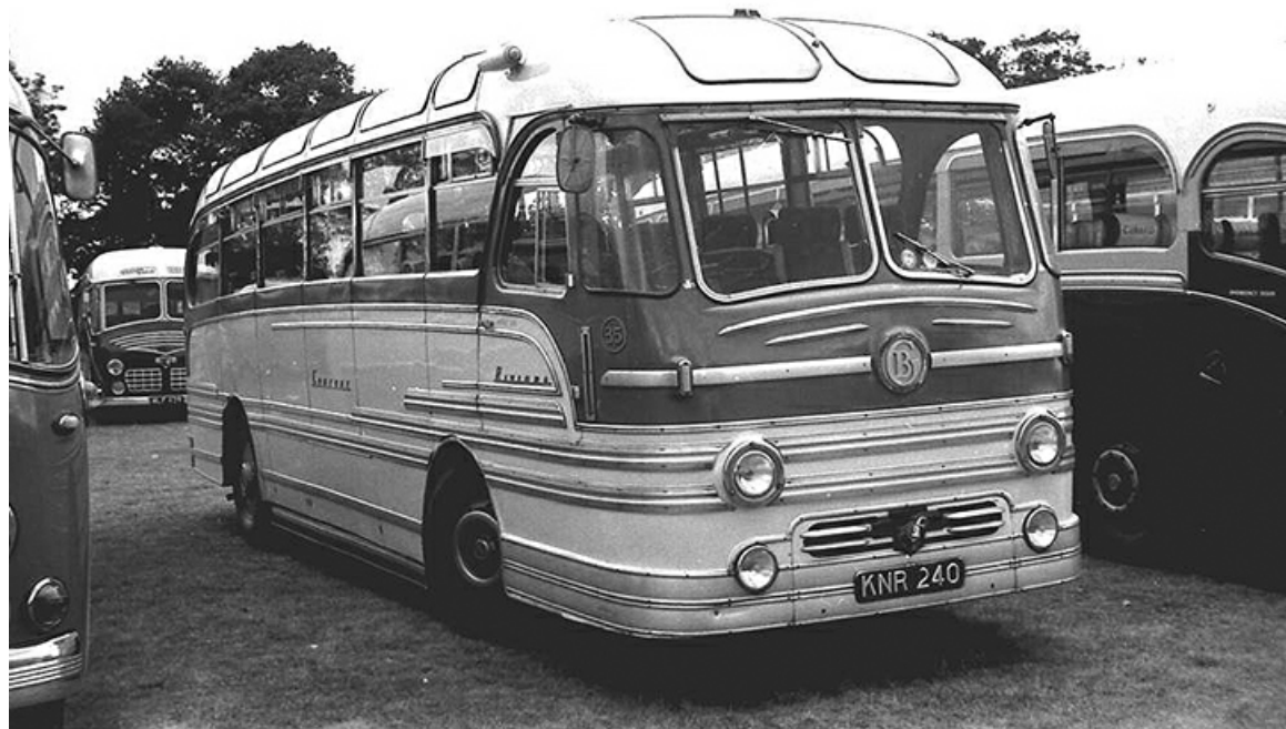
One of two vehicles numbered 35 was KNR240, a Leyland PSU1/13 with Yeates 'Riviera' 41-seat coachwork. (John Boylett courtesy John Kay).
