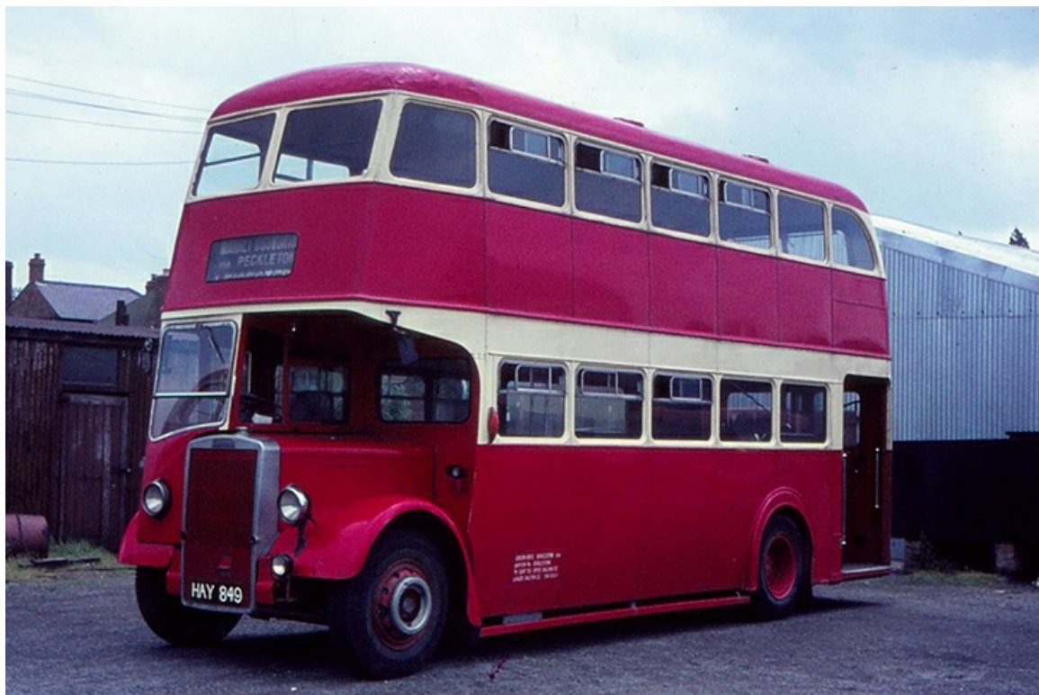
New in 1951 was No. 32(HAY849), a Leyland PD2/12 'Titan' with Leyland 58-seat bodywork. (Stuart Johnson).
