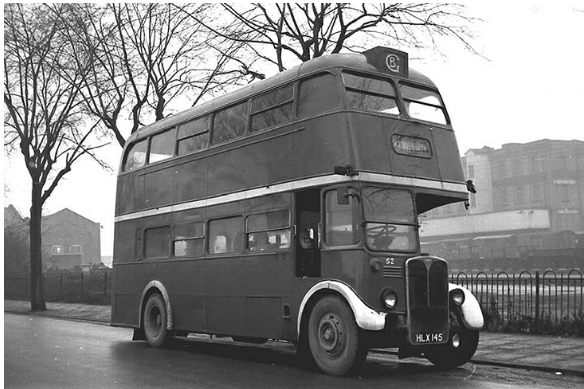
No. 52 (HLX145) was an ex-London Transport RT with Weymann 56-seat bodywork new in 1948 and acquired by Gibson Brothers in 1962. (John Boylett courtesy John Kaye).
