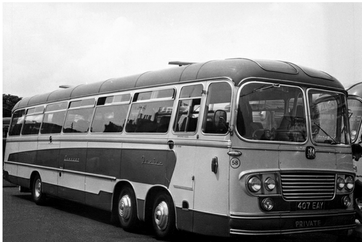
Two six-wheel Bedford VAL14 chassis were added to the fleet in 1963. This is No. 58 (407EAY) with Yeates 52-seat bodywork. (Geoff Stainthorpe).
