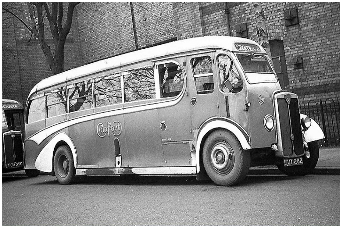
No. 24 (EUT282), was a 1948 Maudslay Marathon III with Willowbrook 33-seat coachwork. (Bus Archive).
