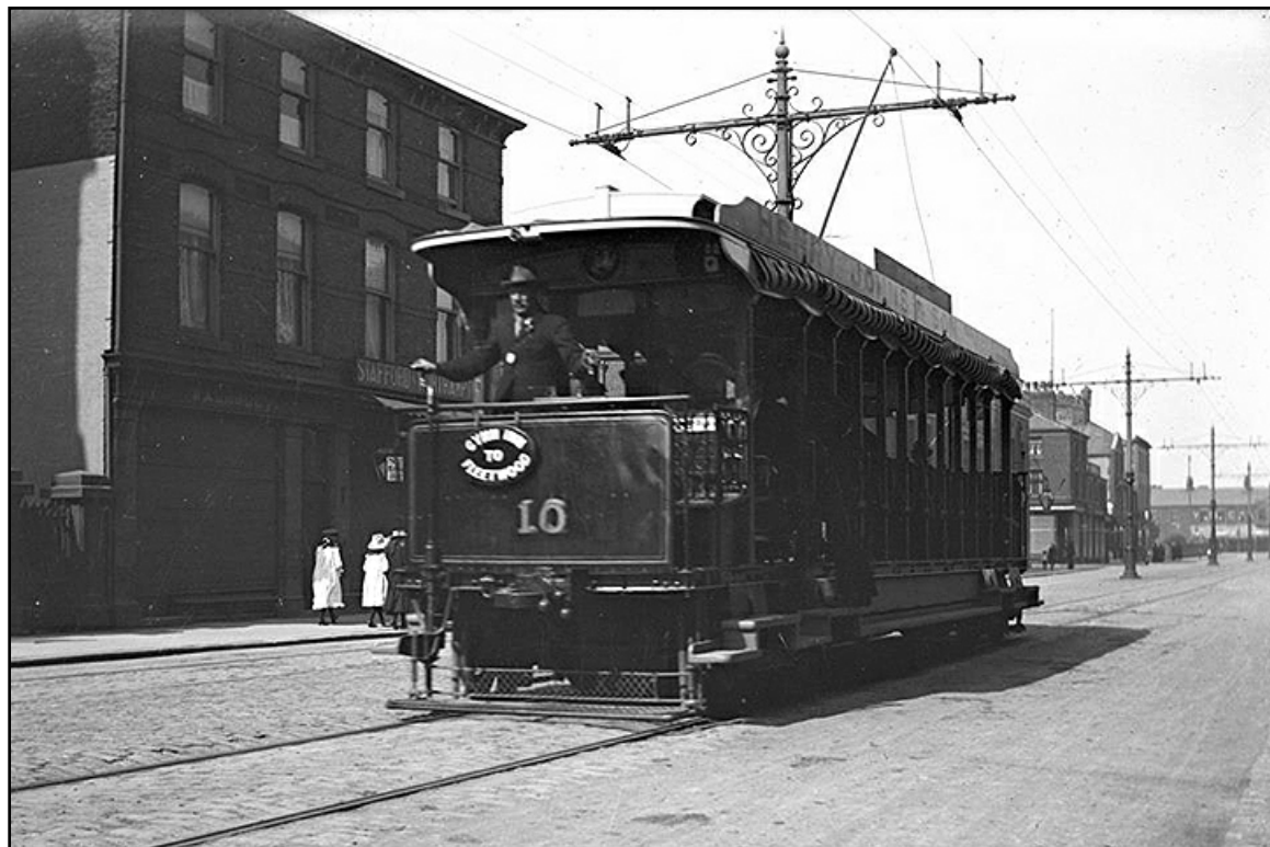
No. 10 was one of the original single-deck covered bogie toastracks purchased by the Company, built by George Milnes & Co it originally seated 48, but were later fitted with crossbench seats on the drivers platform increasing the seating to 56 as seen here. (LTHL collection).
