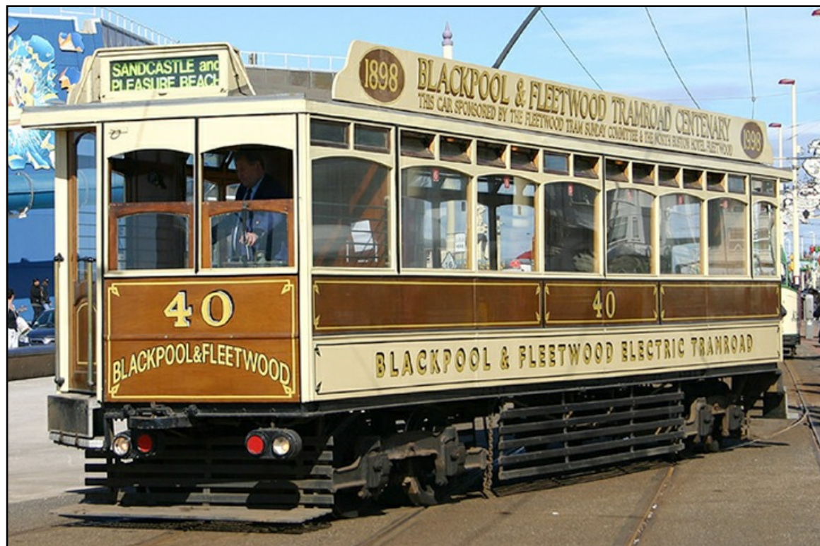
The final delivery of trams in 1914 included No. 40, an enclosed box car with seating for 48 built by the United Electric Car Co of Preston which now survives in preservation. (LTH collection).
