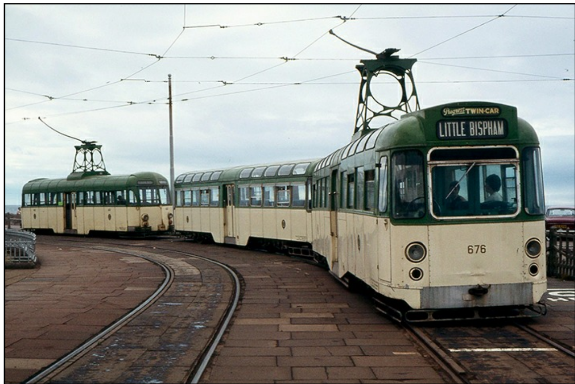
Twin cars were tried by Blackpool during 1958 when No. 276 (later 676) a rebuilt Series 2 Railcoach as seen here was coupled with another rebuilt Railcoach No. 275. (David Flett).
