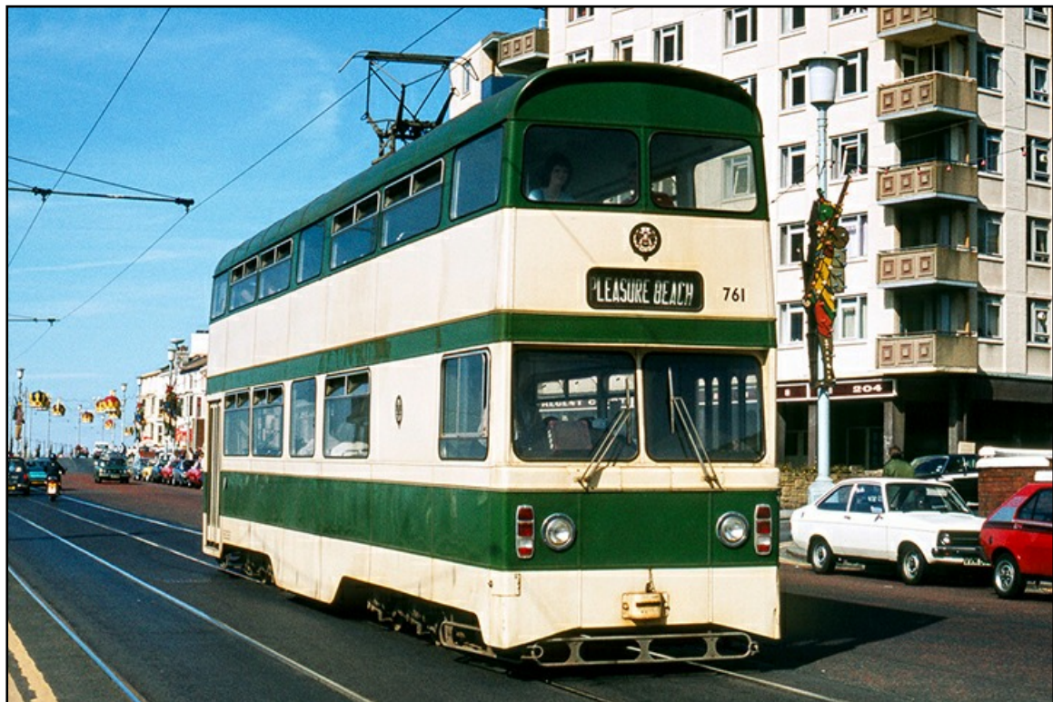
No. 761 was a rebuild of 1935 Balloon car No. 262[725] based on the original teak frame with metal extensions by Metal Sections. It was the first 'Jubilee' car. (David Ingham).
