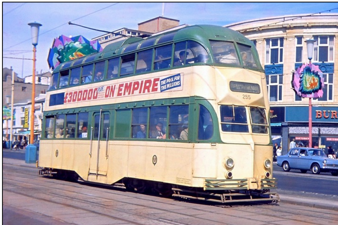
No. 255 was built in 1935 by English Electric and seated 84 passengers. These type of cars gained the nickname 'Balloons' and most were substantially altered during their lifetime. (John Huddleston).
