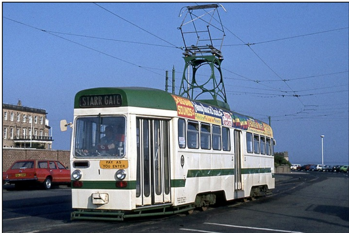
One-man operated car No. 1 was a rebuilt and lengthened 1935 Railcoach No. 269 that entered service in 1972. (LTHL collection).
