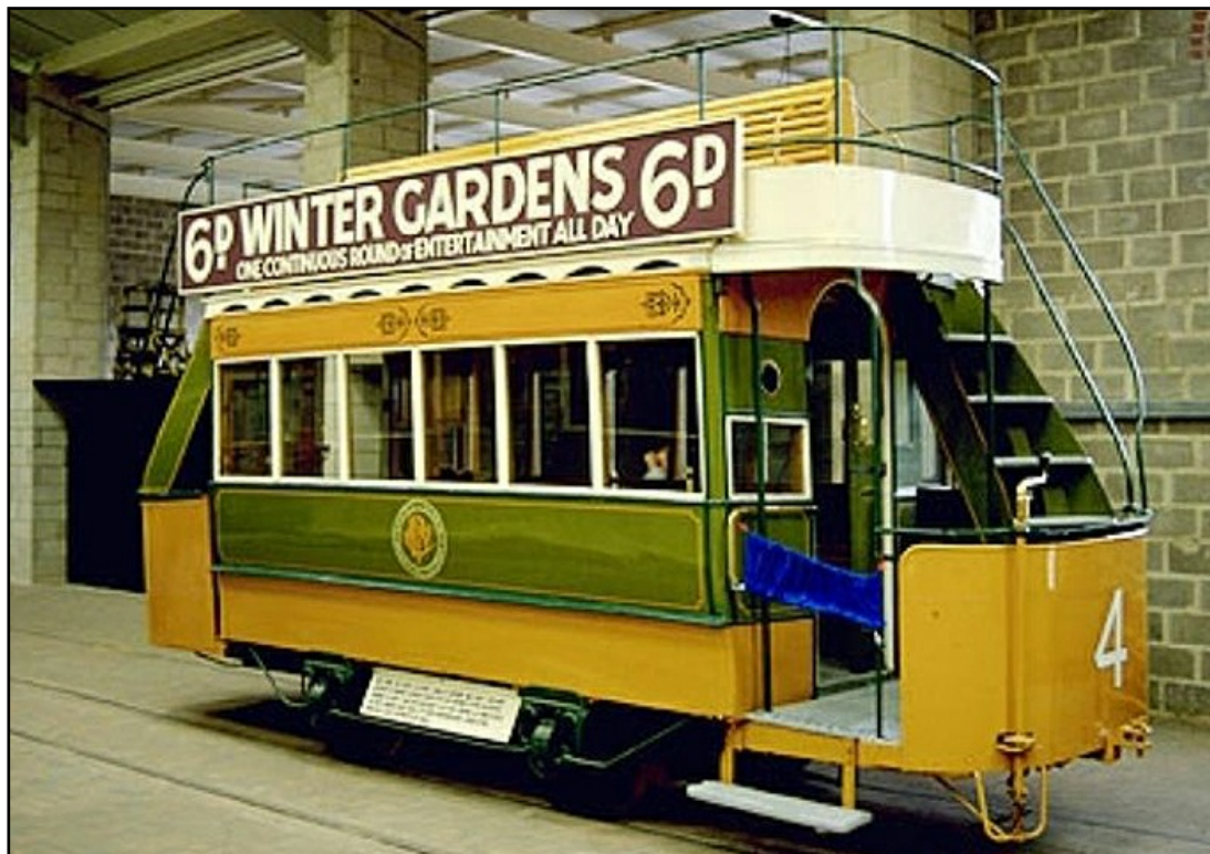
Blackpool Electric Tramway Company's No. 4 was this 32-seat double-deck car built by Lancaster Carriage & Wagon Co in 1885. It survives today at the National Tramway Museum at Crich. (LTHL collection).
