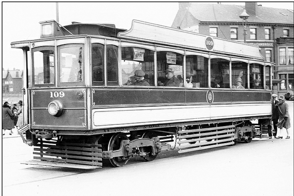
No. 109 was one of the cars acquired from the Blackpool & Fleetwood Tramroad Company in 1920. It was a 1898 Milnes-built saloon fitted with new Preston bogies and upholstered seating by Blackpool Corporation and seated 44. (Blackpool Gazette & Herald).
