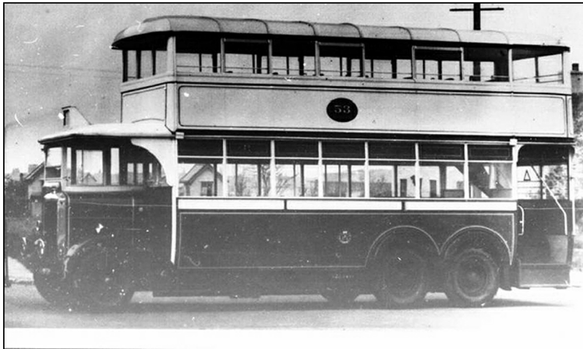
No. 53 (FR8379) was a sole Karrier WL6/2 with Short Bros H30/27R bodywork, new in 1927. It had a relatively short life in the fleet, being withdrawn in 1933. (LTHL collection).
