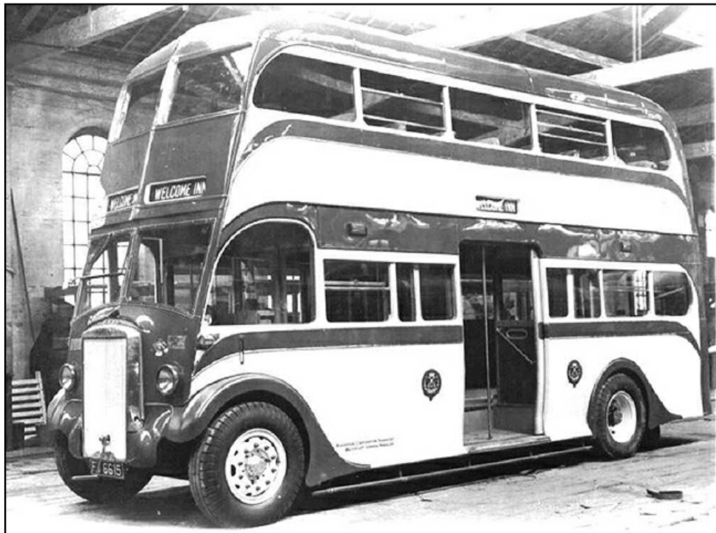
No. 120 (FV6615) was the prototype for the 'Streamline' design introduced in 1935. It was a Leyland TD4 with English Electric 57-seat bodywork. (LTHL collection).
