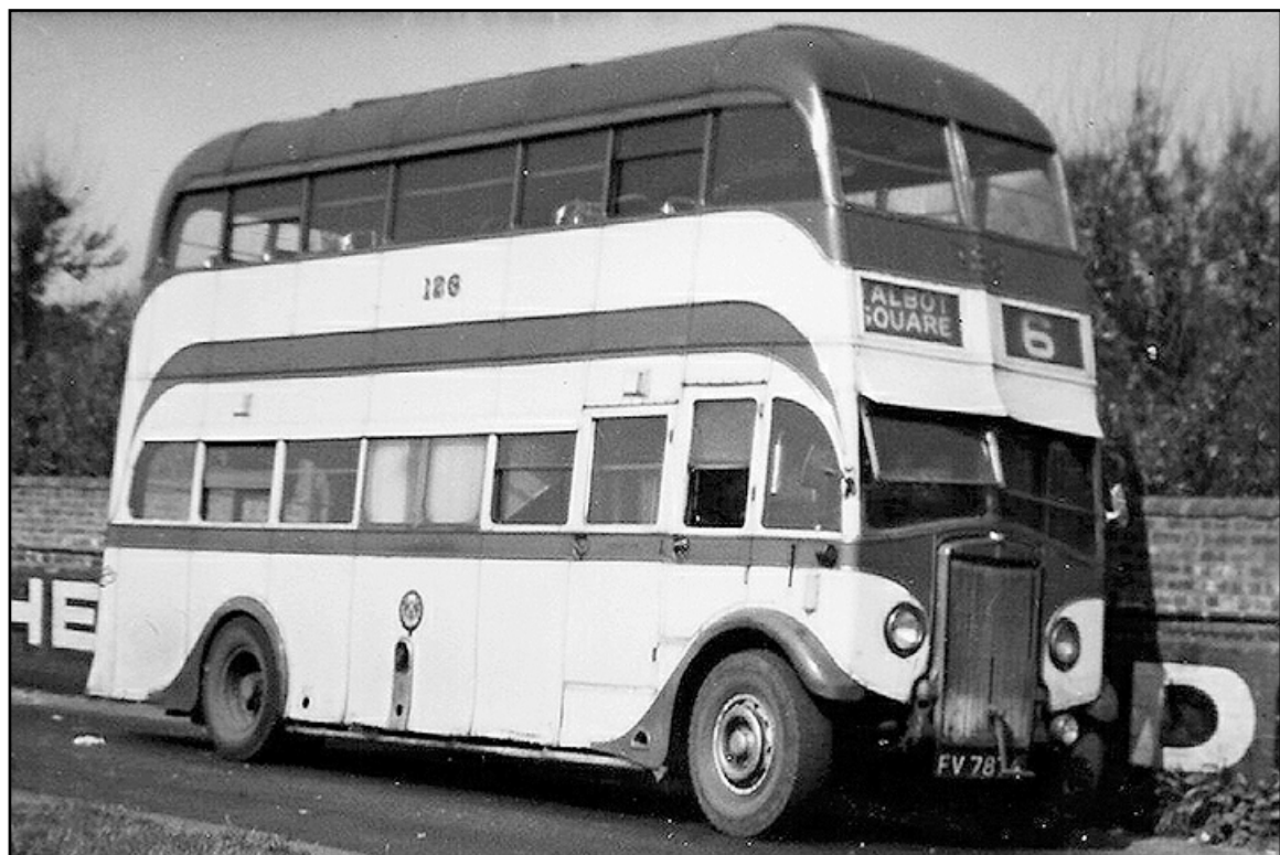
No. 126 (FV7874) was a 1936 Leyland TD4 with Burlingham 48-seat full front bodywork. (Dennis Marshall).
