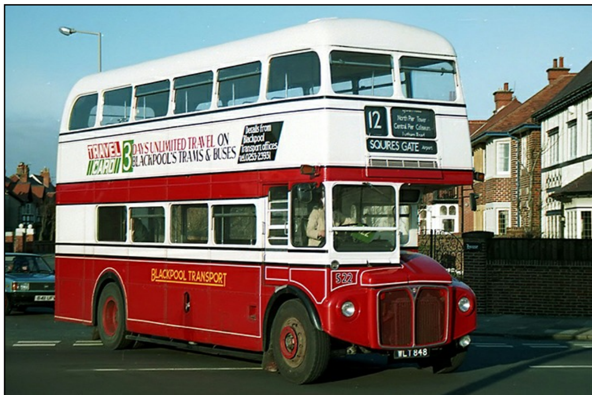
No. 522 (WLT848) was an ex-London Transport 1961 AEC Routemaster with Park Royal H36/28R bodywork. (Joe Gorna11).
