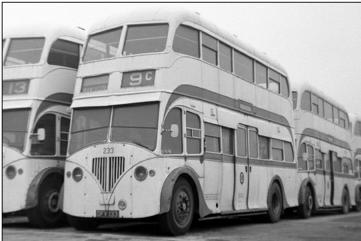
No. 233 (DFV133) was one of fifty Leyland PD2/5s with Burlingham 54-seat 'Streamline' bodywork delivered in 1949. These all had enclosed radiators instead of the exposed radiators on previous models. (LTHL collection).
