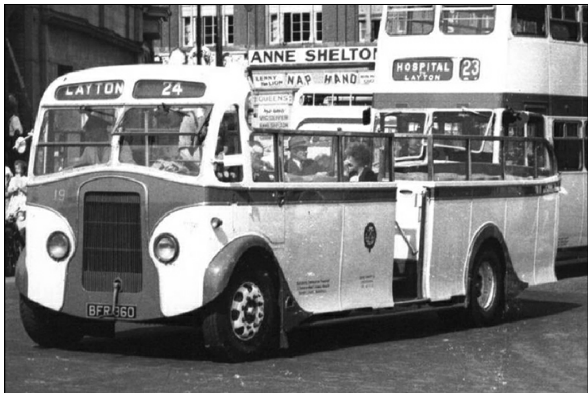
No. 19 (BFR360) was a Leyland LZ2A 'Cheetah' with Burlingham 34-seat open-top bodywork. (LTHL collection).
