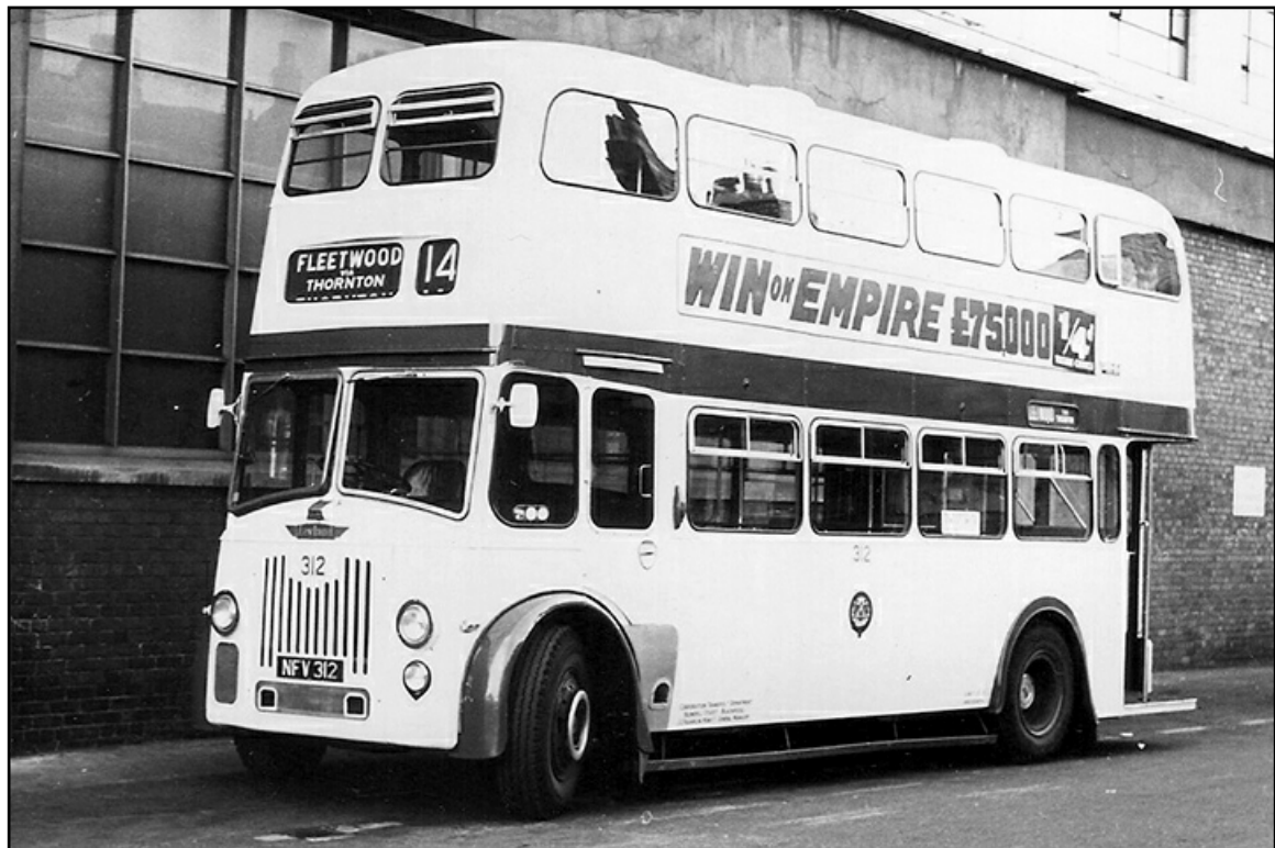
No. 312 (NFV312) was a 1958 Leyland PD2/27 with Metro-Cammell FH35/28R bodywork. (LTHL collection).
