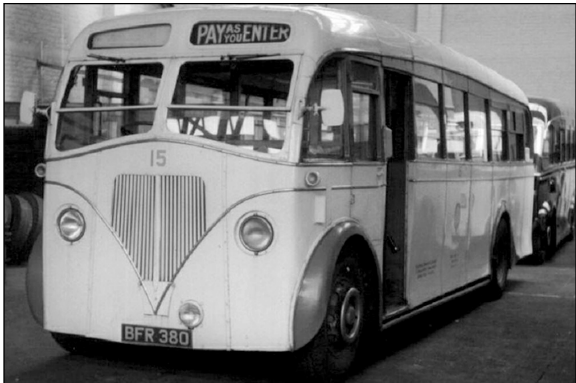
No. 15 (BFR380), a 1940 Leyland TS8 'Tiger' originally had a centre entrance but was converted to forward entrance as seen here in 1955 for PAYE operation. (LTHL collection).
