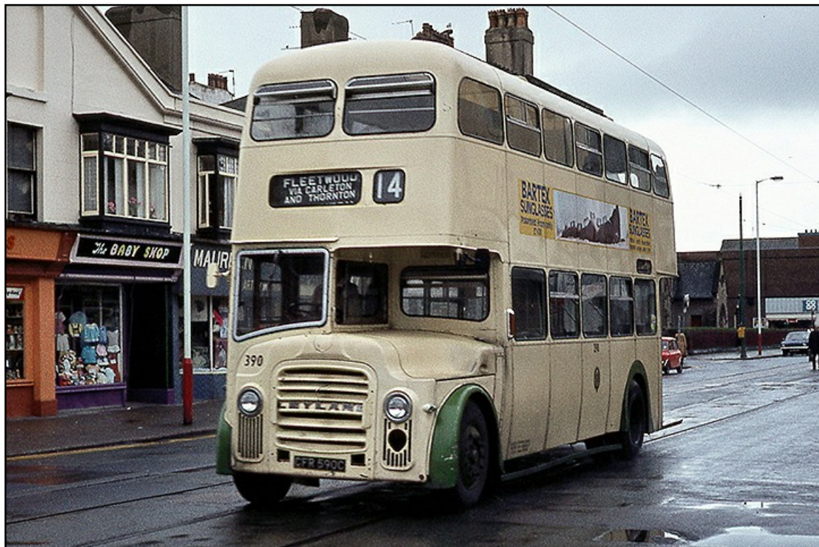
No. 390 (CFR590C), a 1965 Leyland PD3A/1 'Titan' with Metro-Cammell H41/30R bodywork, making its way to Fleetwood on a rainy day in Blackpool. (David Flett).
