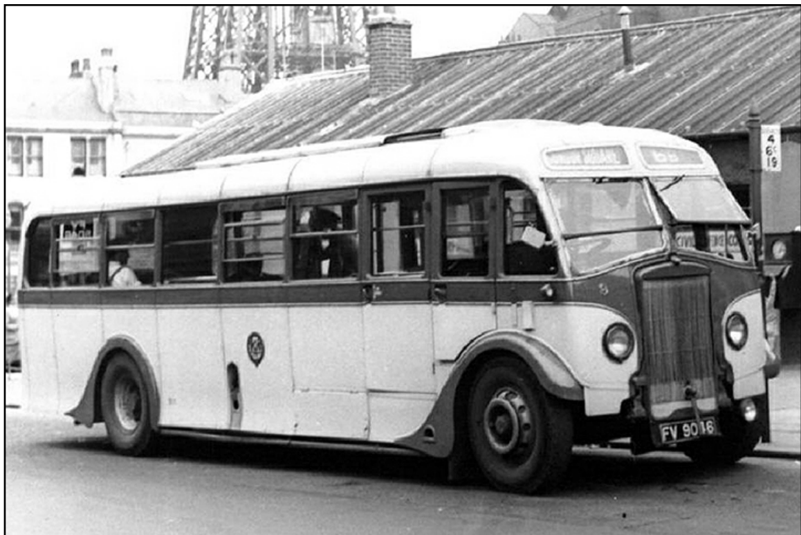
No. 9 (FV9046) was a 1937 Leyland TS7 with Burlingham 34-seat full front bodywork. (LTHL collection).
