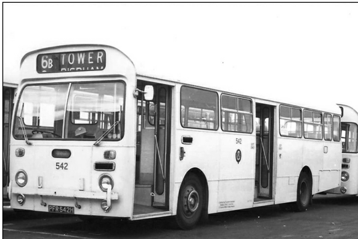
No. 542 (PFR542H), a 1969 AEC Swift with Marshall dual door 47-seat bodywork. (LTHL collection).
